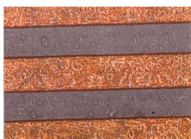
Figure 25 – Board surface at the best dew formation condition
