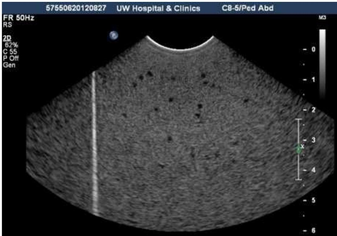
Figure D.2 – Image obtained by using the phantom containing 2 mm-diameter, low-echo spheres and a pediatric transducer with a radius of curvature of about 1,5 cm
