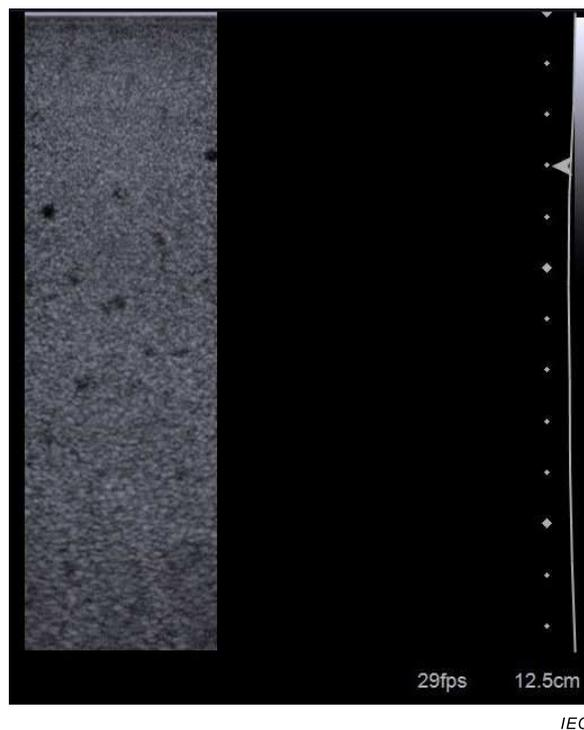
Figure C.1 – One image obtained from a phantom containing 3,2 mm-diameter, low-echo spheres by using a 4 MHz linear array focused at 3 cm
