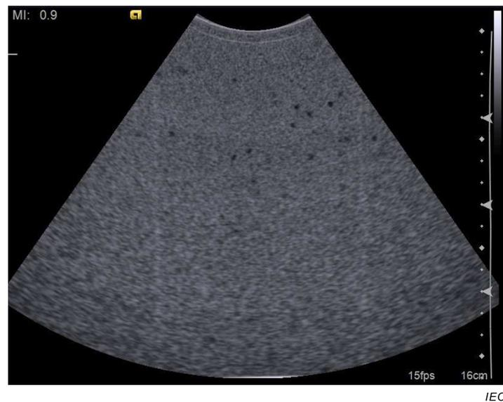
**Figure C.4 – Sector image (curved array) at 4,5 MHz with multiple foci at 4 cm, 8 cm and 12 cm depths; the low-echo spheres are 3,2 mm in diameter**
