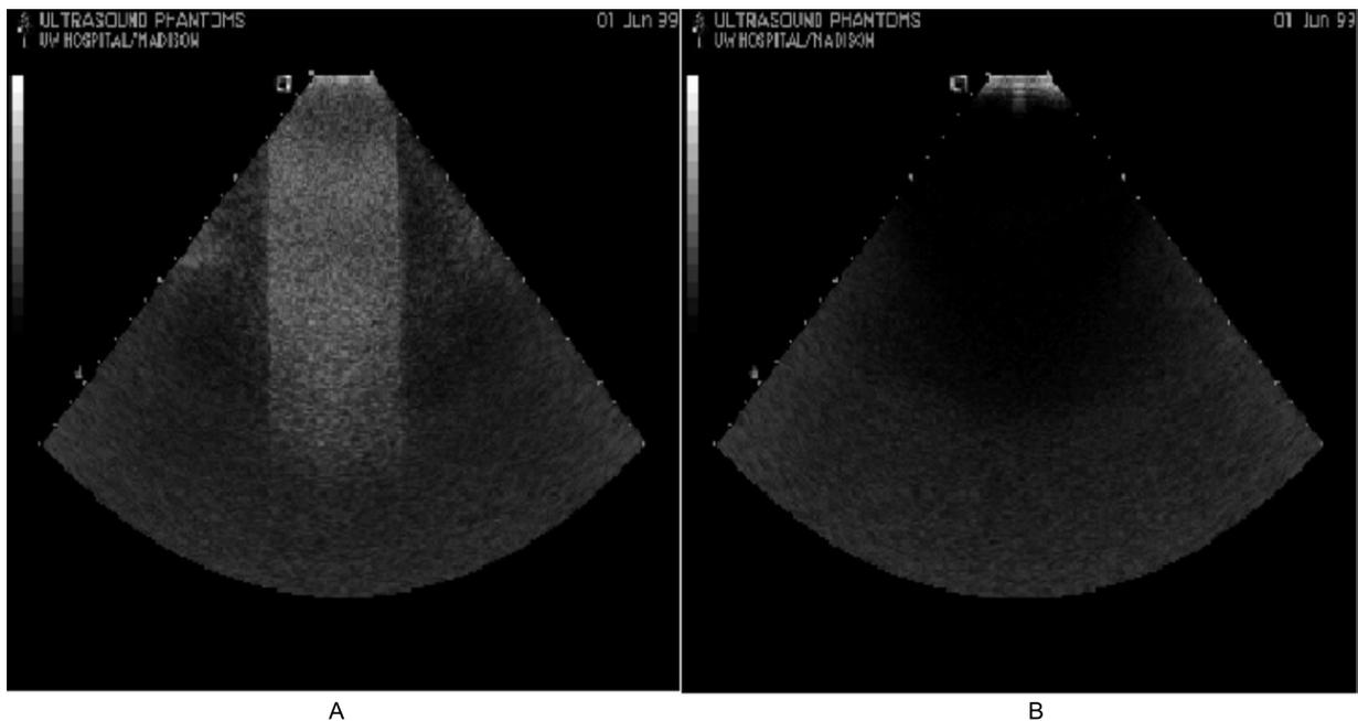
**Figure 2 – A) Image of a uniform section in a tissue-mimicking phantom, bright rectangle; B) Image displaying electronic noise only, obtained with the operating controls set the same as for A but with the transducer decoupled from the phantom [SOURCE: University of Wisconsin]**
