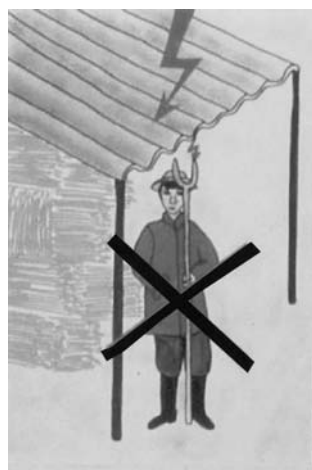
Figure 4 – Unsuitability of metallic structures when not earthed
