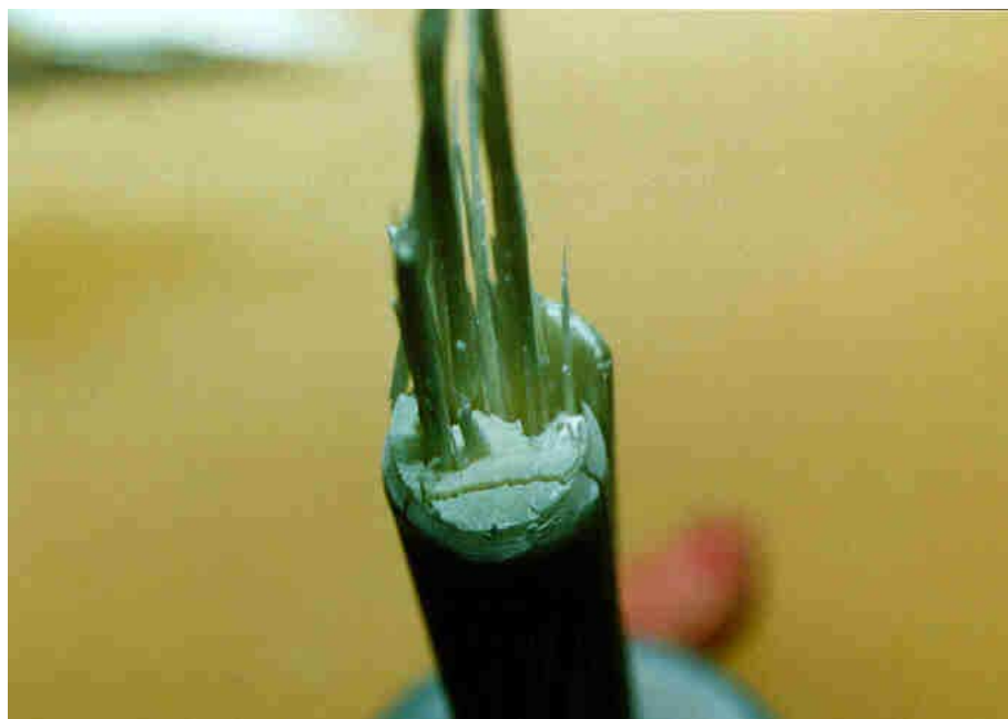
Figure 1 – Typical brittle fracture
