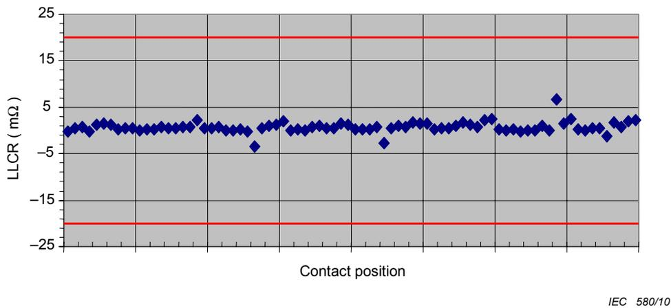
**Figure 27 – Change in the LLCR due to electrical and mechanical discharge for IEC 60603-7 connectors including 2 m, 10 m, and 100 m cables combined**
