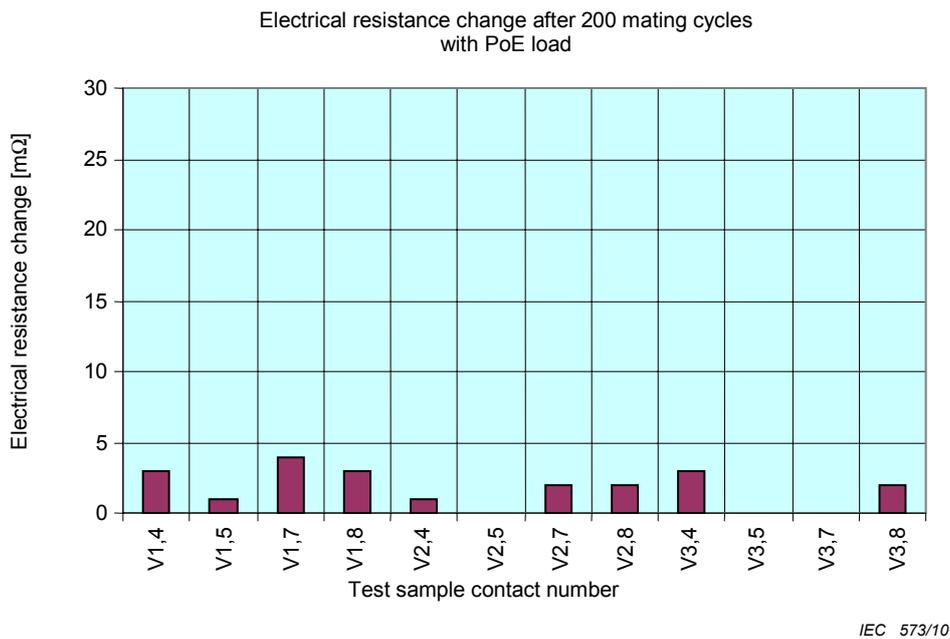
Figure 20 – Test results test 6A
