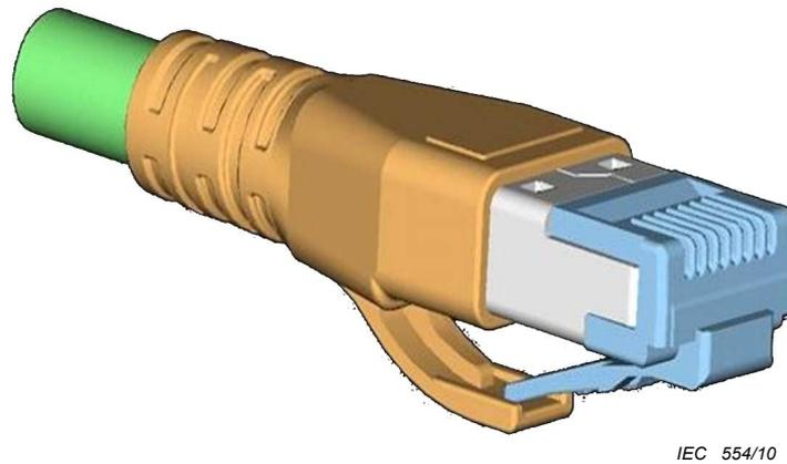
Figure 1 – Illustration of a typical shielded 8-way connector according IEC 60603-7
