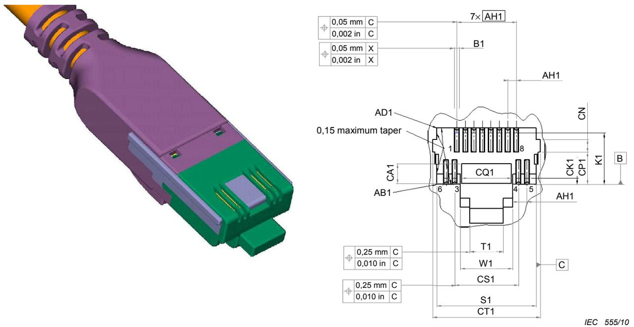
Figure 2 – Illustration of an IEC 60603-7-7 or IEC 61076-3-110 connector
