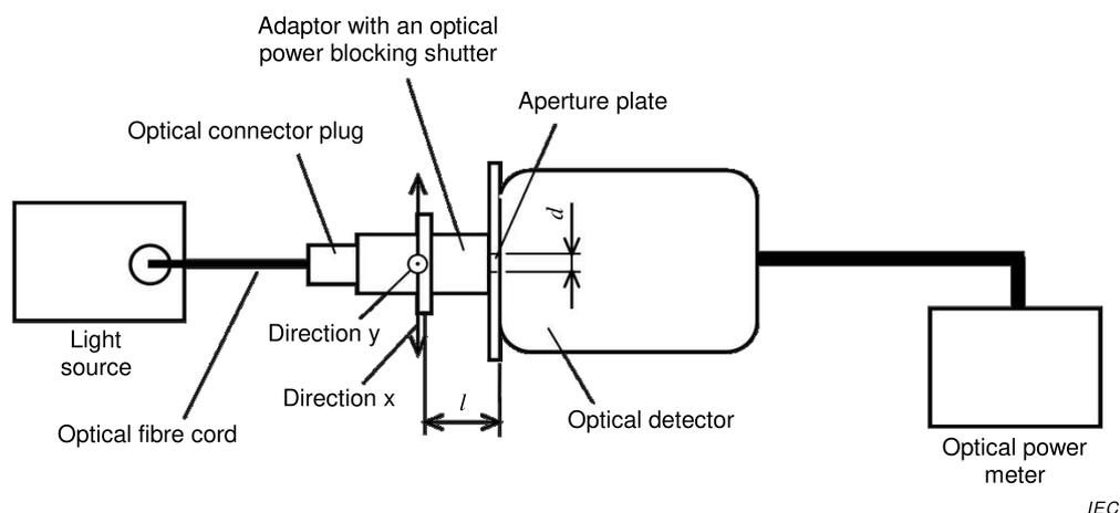
**Figure 2 – Example of measurement set-up for Method 2**
