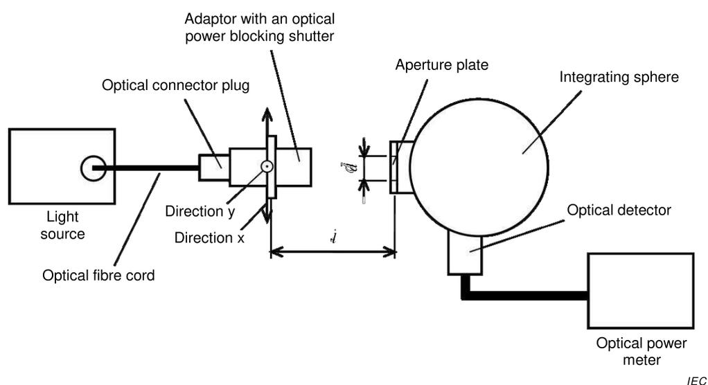
**Figure 1 – Example of measurement set-up for Method 1**
