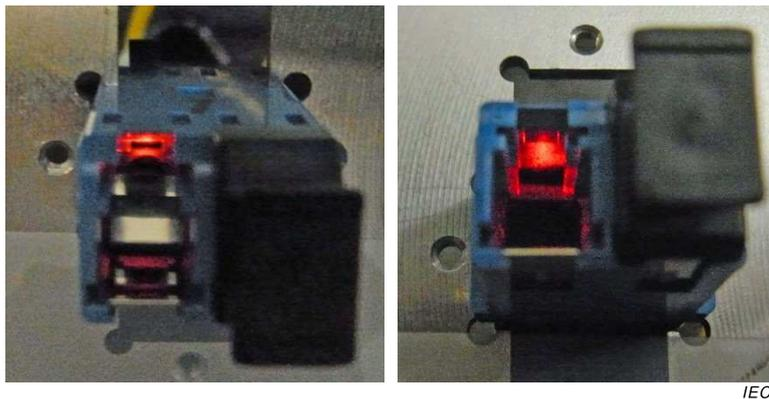
**Figure A.1 – Example of off-axis emitted visible light
