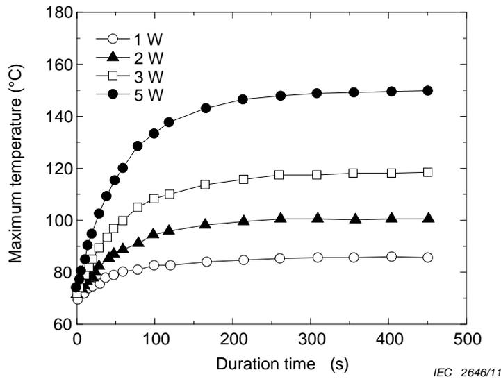
**Figure 10 – Maximum internal temperature of optical splitter by thermal simulation (forward direction, input power: 5 W)**
