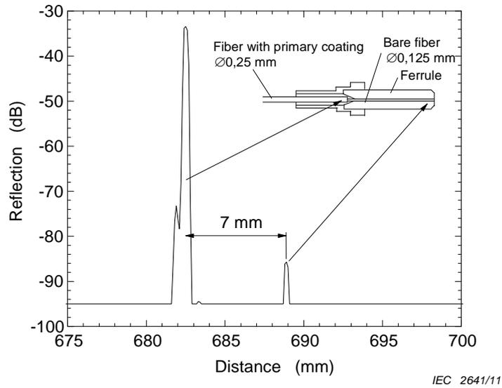
Figure 5 – Measurement result for the ferrule point of reflection in the optical isolator
