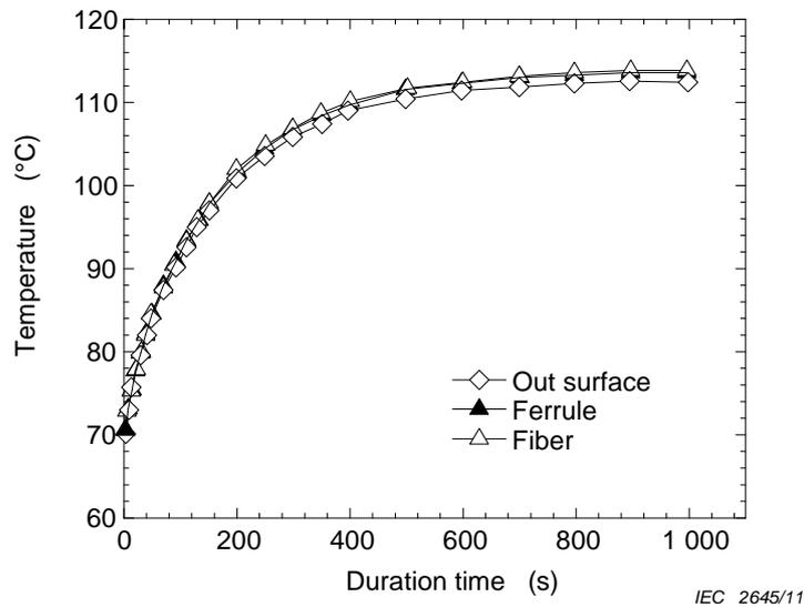
Figure 9 – Thermal simulation of optical isolator (forward direction, input power: 5 W)
