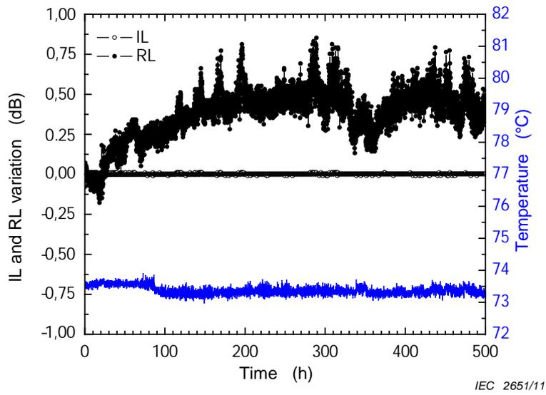
Figure 14 – Change of IL and RL of optical isolator
