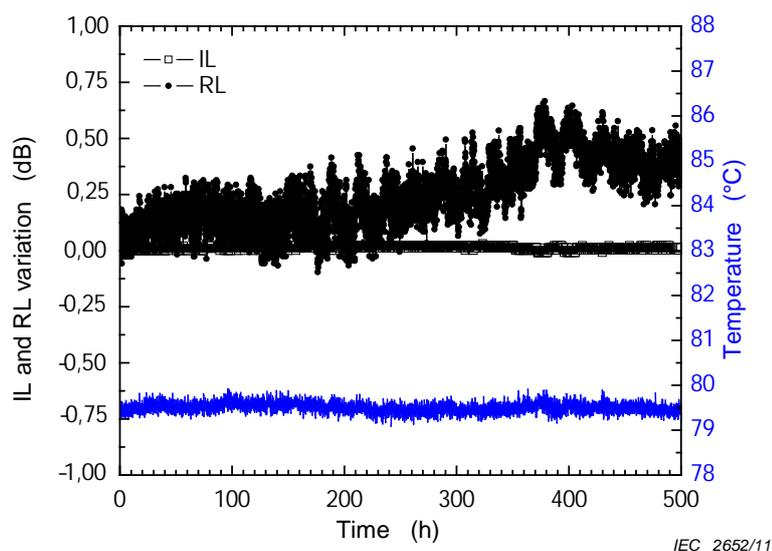
**Figure 15 – Change of IL and RL of optical splitter**
