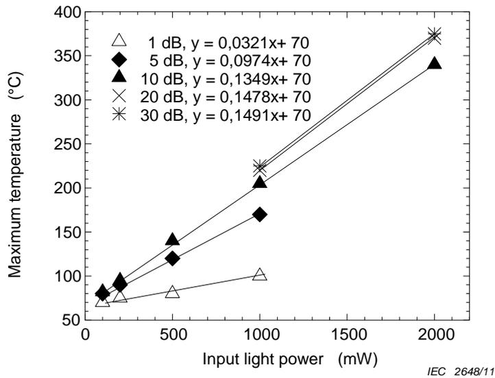
Figure 12 – Relationship between input light power and maximum temperature in the thermal simulation of fixed optical attenuator
