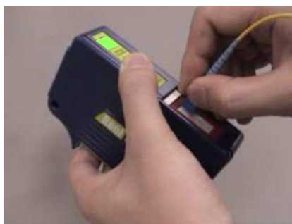
Figure 7 – Cleaning with a reel type cleaner
