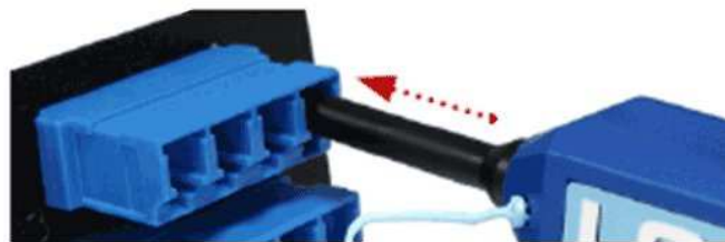
Figure 9 – Cleaning ports using a pen type cleaner
