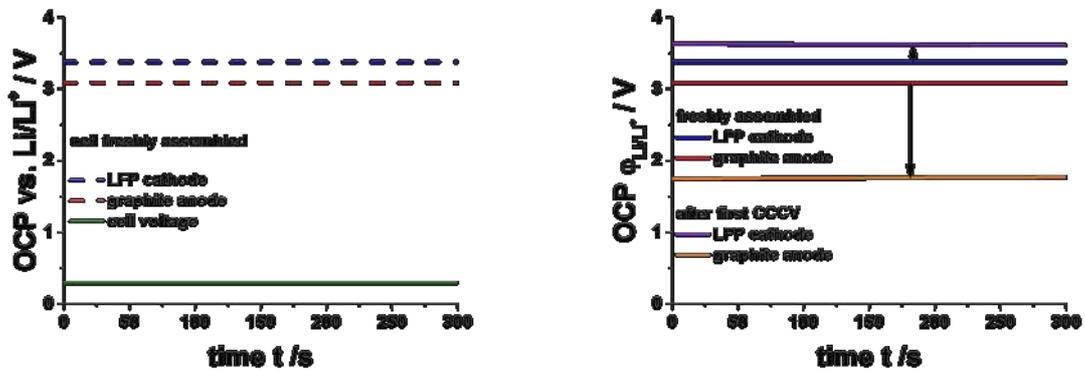
a) Open circuit potential of LFP cathode and graphite anode for freshly assembled cell
