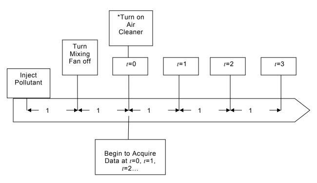
For dust, obtain at least 9 data points (over 20 min). For pollen, obtain at least 5 data points (over 10 min). For natural decay, do not turn on air cleaner\*, and begin data acquisition at t = 0.
