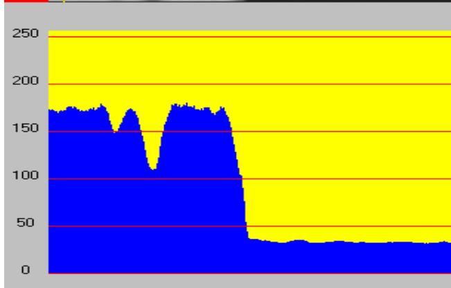
Grey scale profile showing the disconnected elements as smaller and larger wedges and on the right side loss of sensitivity of elements.
