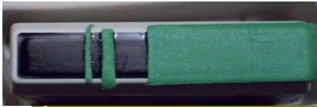
Transducer covered with small strips of tape (5 layers) to simulate disconnected elements. The larger piece of tape simulates loss of sensitivity.
