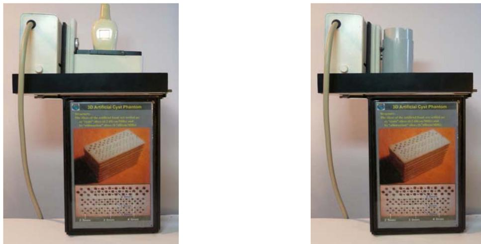
Figure A.7 – Phantom with motor drive and two types of adapters
