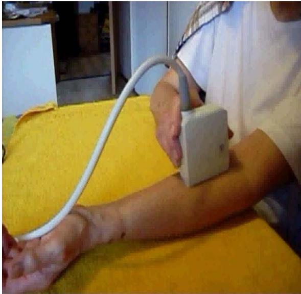
**Figure D.1a) – Uniformity test with related linear or curved array transducer**
