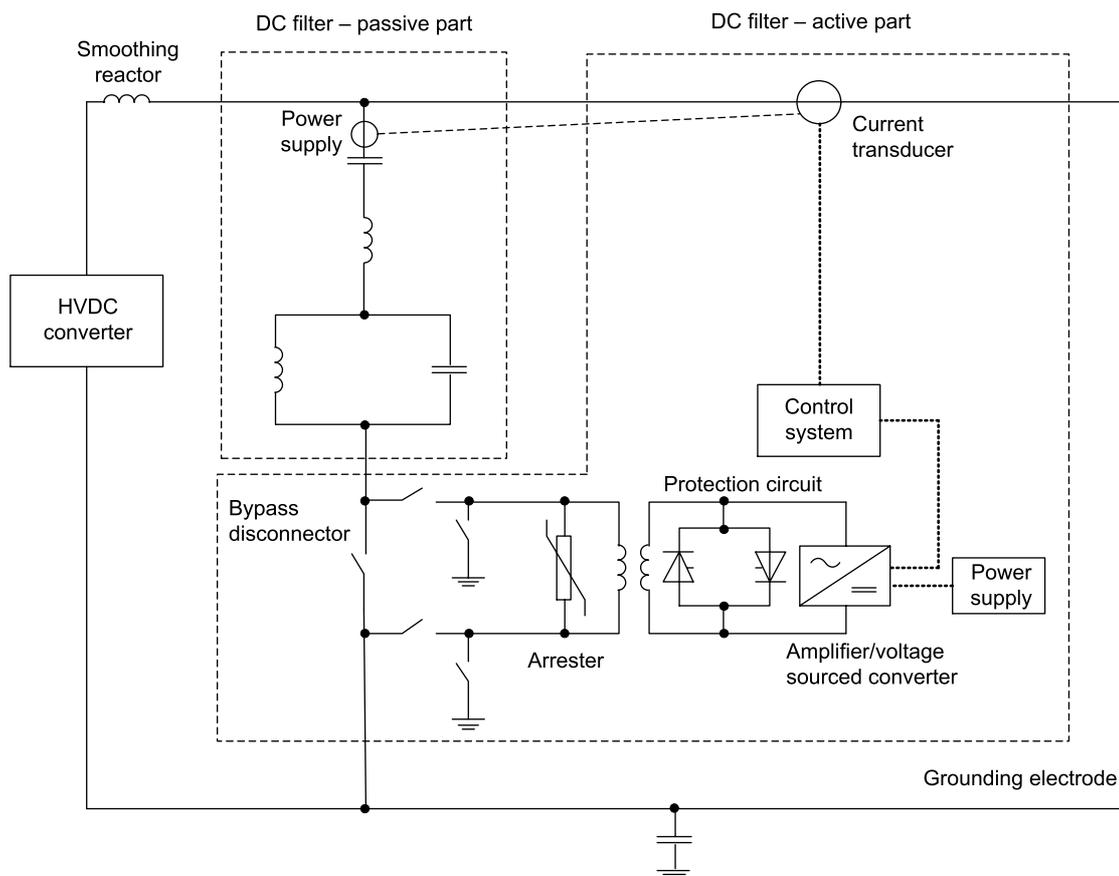
Figure 7 – Filter components in the active filter
