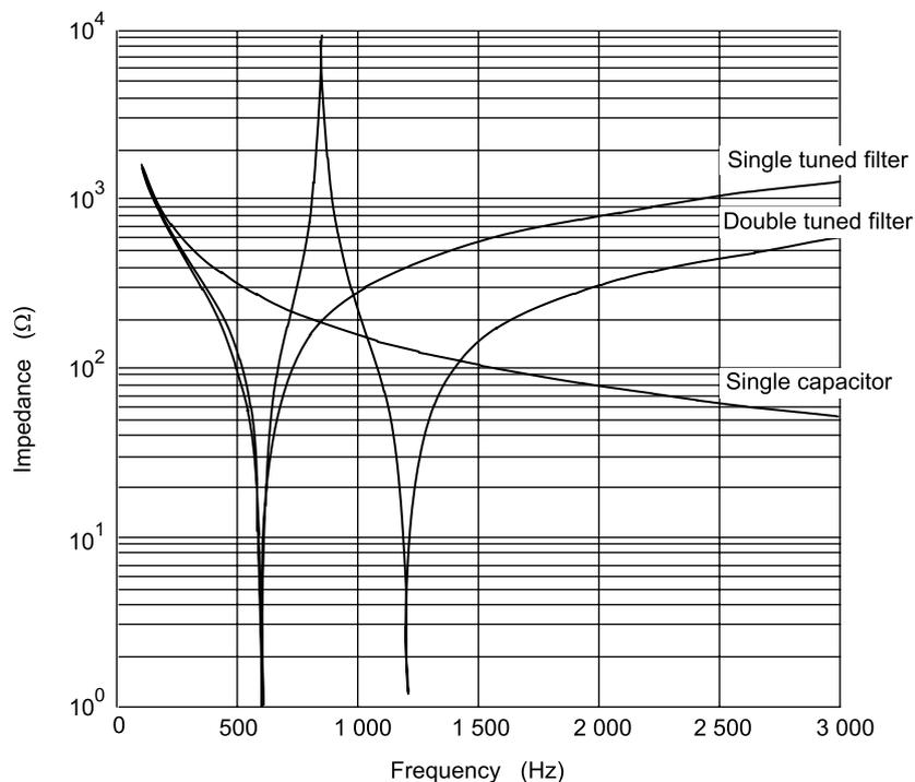
Figure 8 – Impedance characteristics of different passive filters
