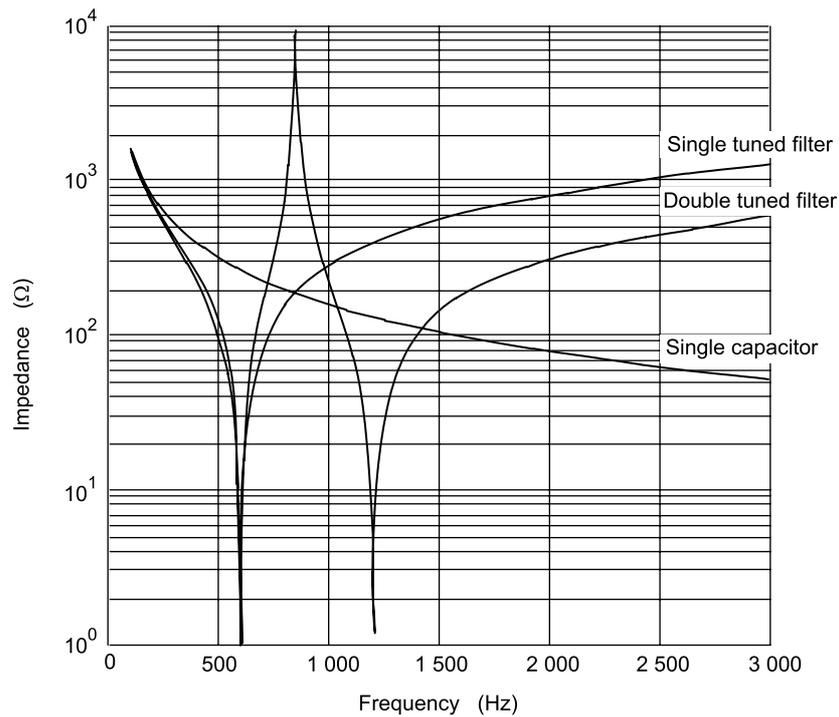
**Figure 8 – Impedance characteristics of different passive filters** IEC 1827/11
