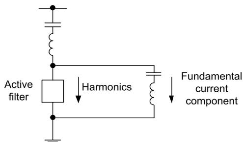
Figure 23 – Using an LC circuit to divert the <sup>IEC 1842/11</sup> fundamental current component
