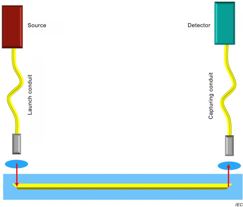
**Figure 7 – Measurement setup with orthogonal launch and capture direction**
