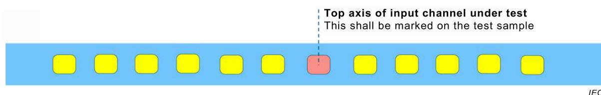
4 a) Cross-sectional front view of the input facet of the channel under test
