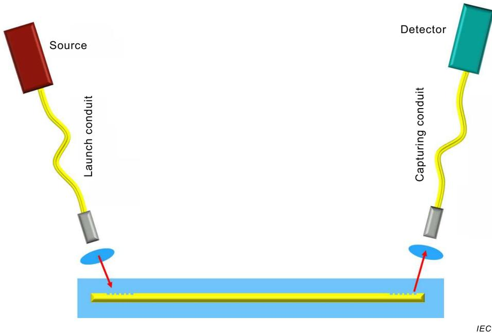
**Figure 8 – Measurement setup with oblique launch and capture direction**
