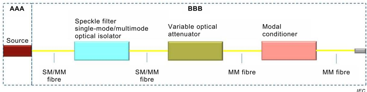
**Figure 3 – Recommended test setup for multimode fibre launch conditions**
