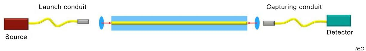
**Figure 6 – Measurement setup with collinear launch and capture direction**
