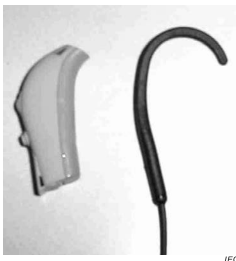
Figure 1 – An ear-hook induction transducer, with a BTE (behind the ear) hearing aid body for scale
