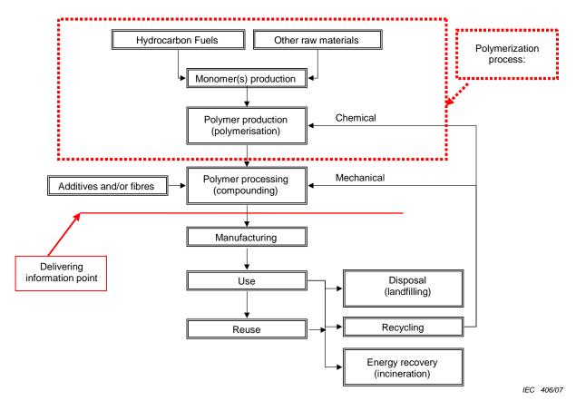
The analysis should be focusing on the compounding process and its environmental aspects (see Figure 1).
