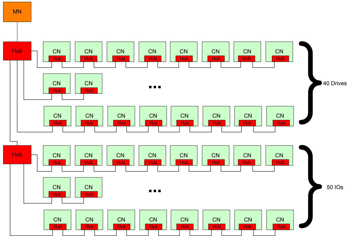
Figure 105 – EPL V2.0 Timing Example 4 (40 drives and 50 IO's)
