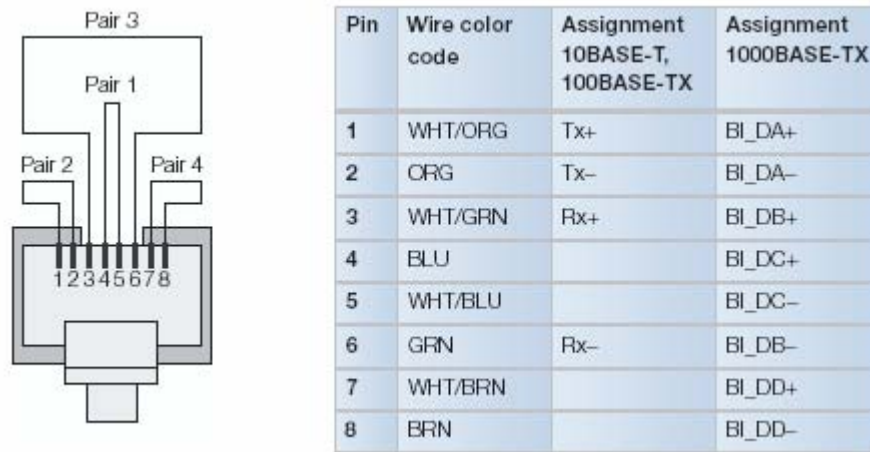
Figure 13 – RJ45 pin assignment
