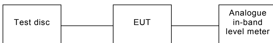
Figure 4 – Block diagram for audio output level measurement
