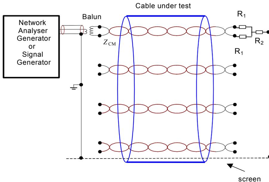
**Figure 3 – Termination of the cable under test**
