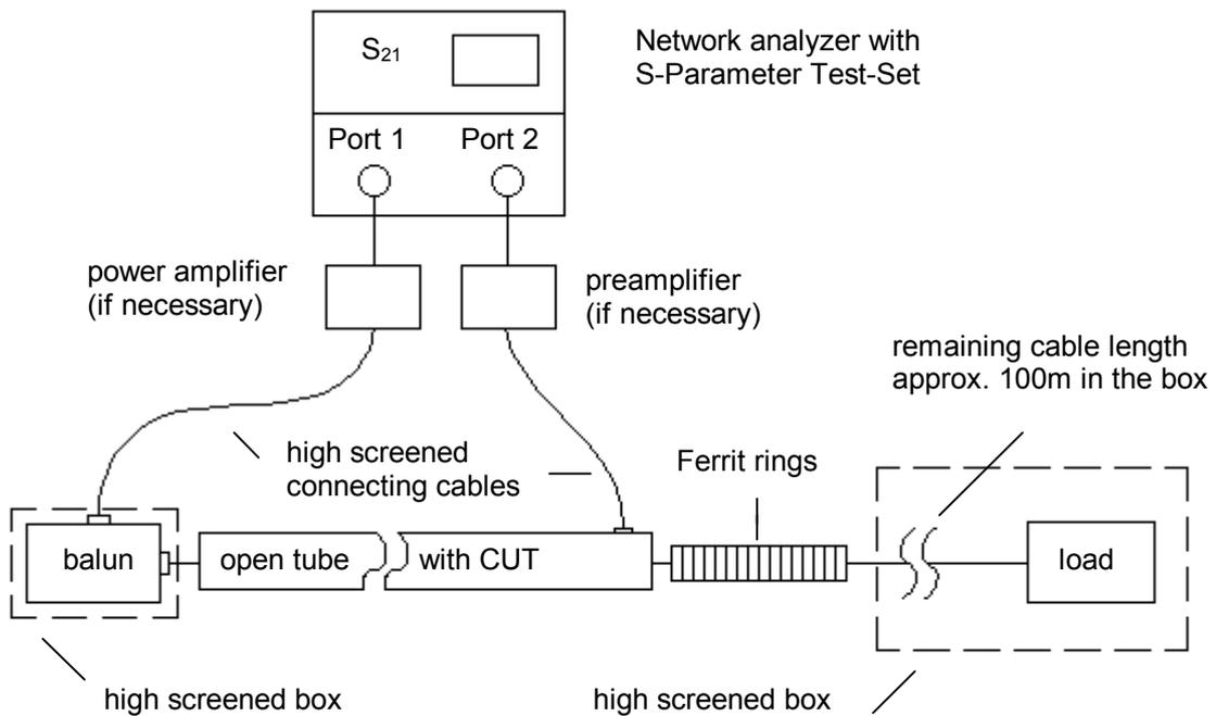
Figure 2 – Set-up to measure the coupling attenuation
