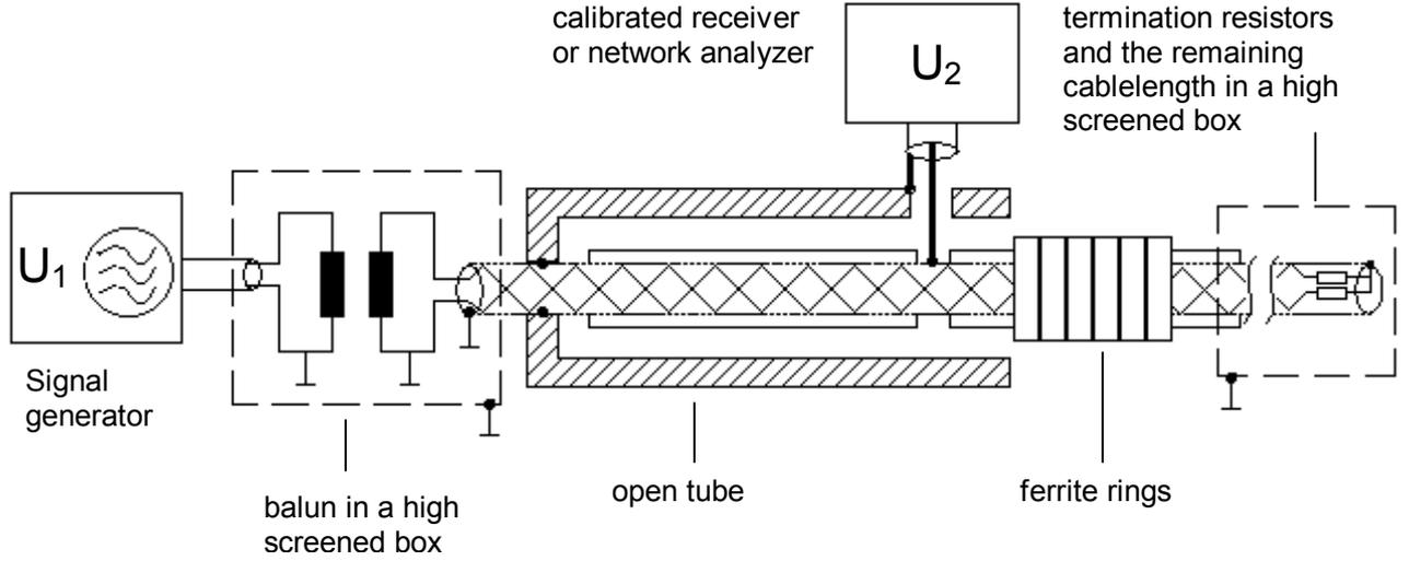
Figure 1 – Principle test set-up
