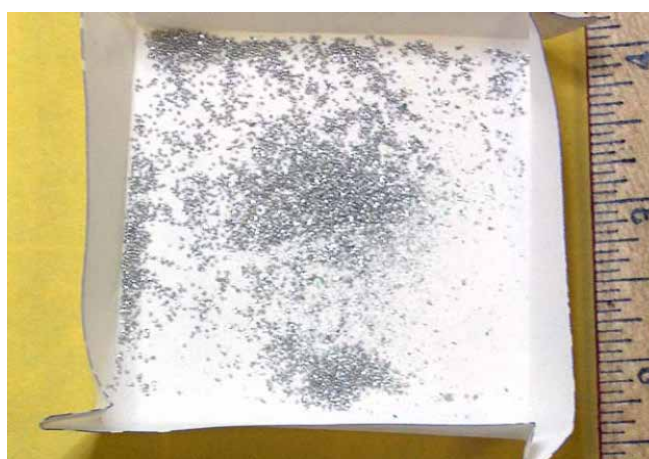
Figure E.12 – Solder ball material collected from BGA using a hand removal procedure
