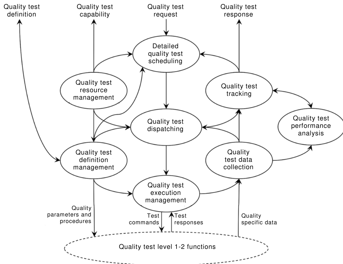
Figure 22 – Activity model of quality test operations management
