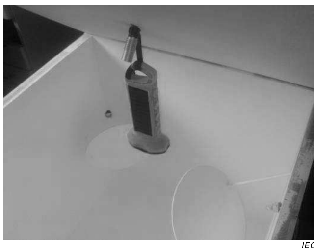
Figure M.1 – Interior view of photometer box with suspended light
