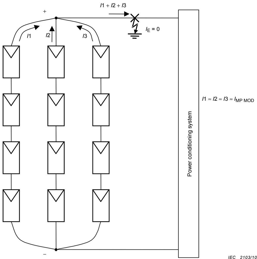
**Figure F.2 – Floating PV array with single earth fault**
