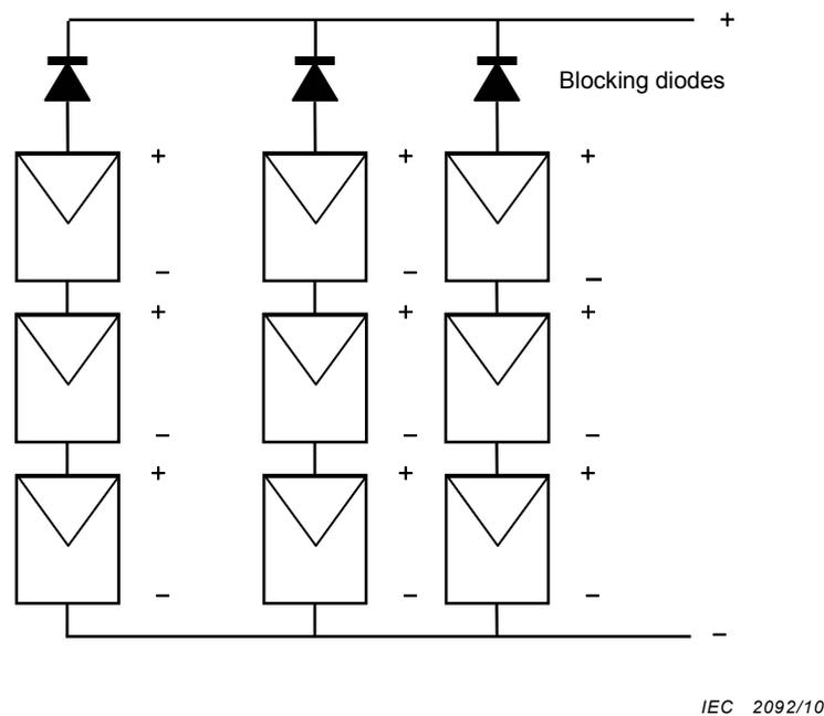
**Figure 14 – Blocking diode implementation (example)**
