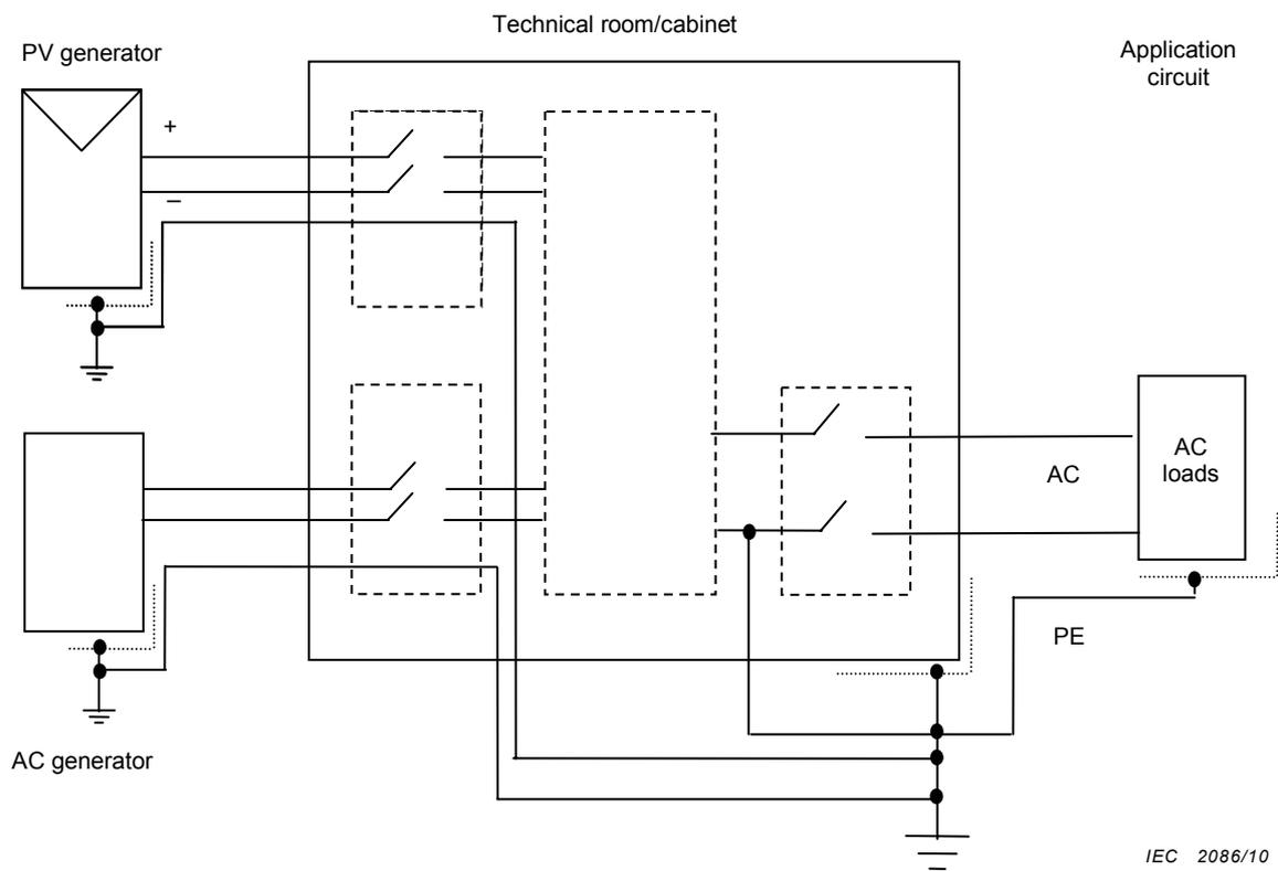
**Figure 8 – Configuration D and F – Hybrid IES or CES – PV generator + inverter and other generator –  $d < 15$  m**
