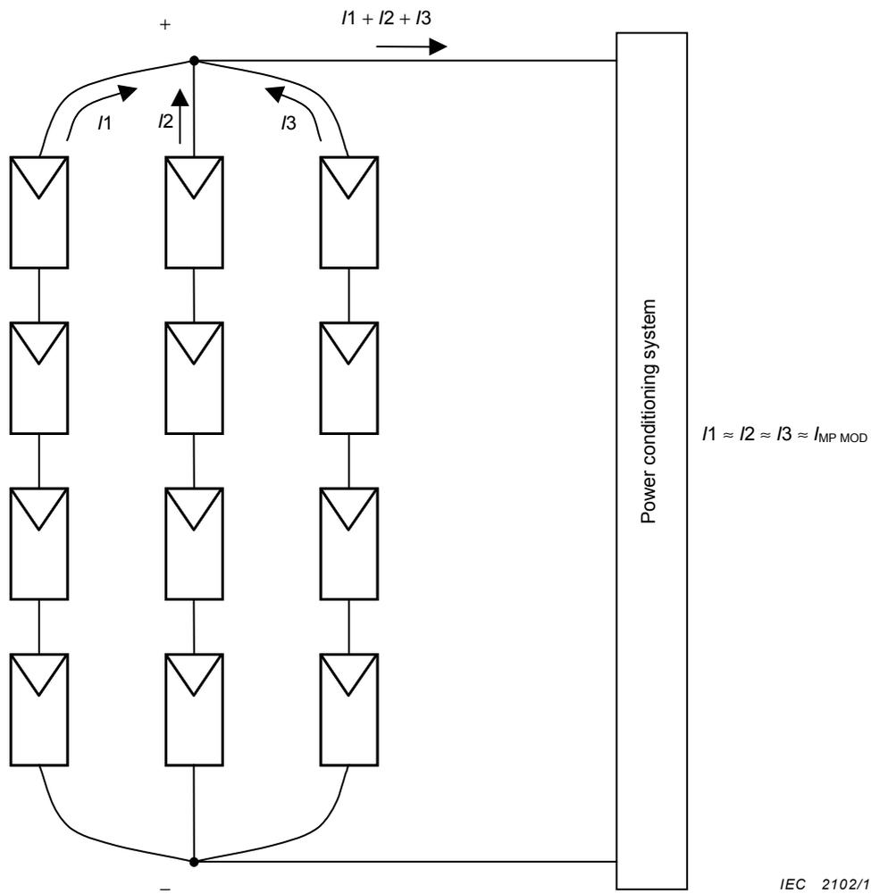
**Figure F.1 – Floating PV array operating at maximum power point**
