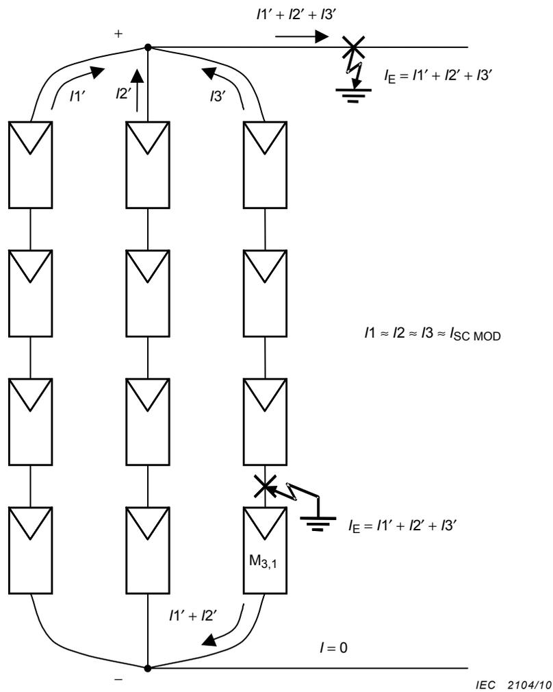
**Figure F.3 – Floating PV array with double earth fault**
