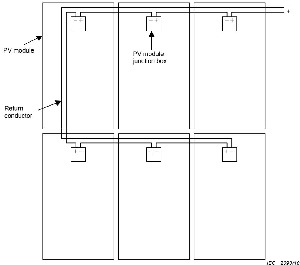
Figure 15 – PV string wiring with minimum loop area
