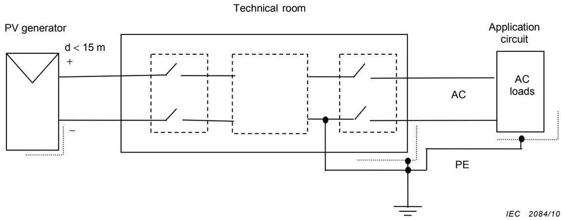
**Figure 6 – Configuration C and E – PV alone IES or CES –  $P < 500\text{ W}$  – with inverter –  $d < 15\text{ m}$**
