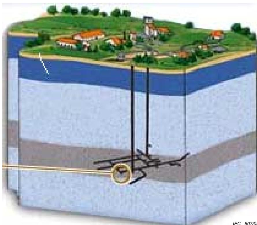
**Figure 9 – French underground laboratory for studies in clay storage of long-lived high level waste (HLW-LL)**
