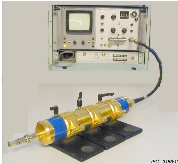
**Figure 73 – TDR test setup**
