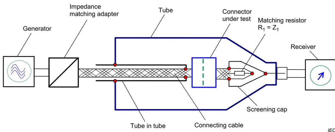
**Figure 7 – Measuring the screening attenuation with tube in tube with impedance matching device**
