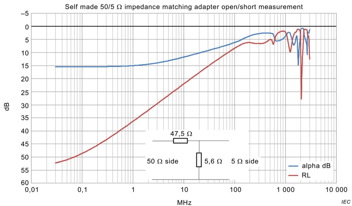
**Figure B.1 – Attenuation and return loss of a 50  $\Omega$  to 5  $\Omega$  impedance matching adapter, log scale**
