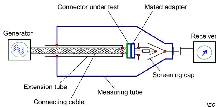
**Figure C.8 – Triaxial set-up with extension tube for connectors**
