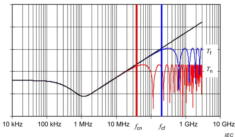
**Figure C.3 – Calculated coupling transfer function ( $l = 1 \text{ m}$ ;  $\epsilon_{r1} = 2,3$ ;  $\epsilon_{r2} = 1$ ;  $Z_F = 0$ )**
