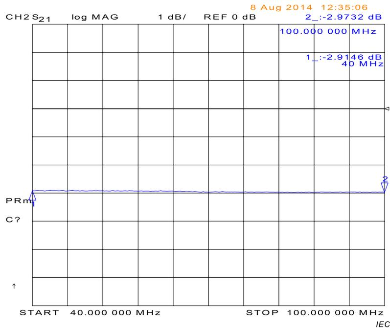
Figure E.1 – Measurement with HP8753D of  $S_{21}$  of a 3dB attenuator
