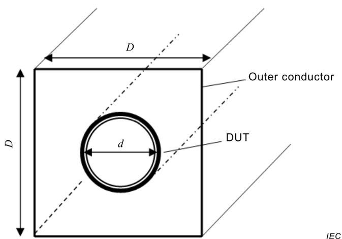
**Figure G.2 – DUT with uniform cylindrical shape in the centre of the cell**
