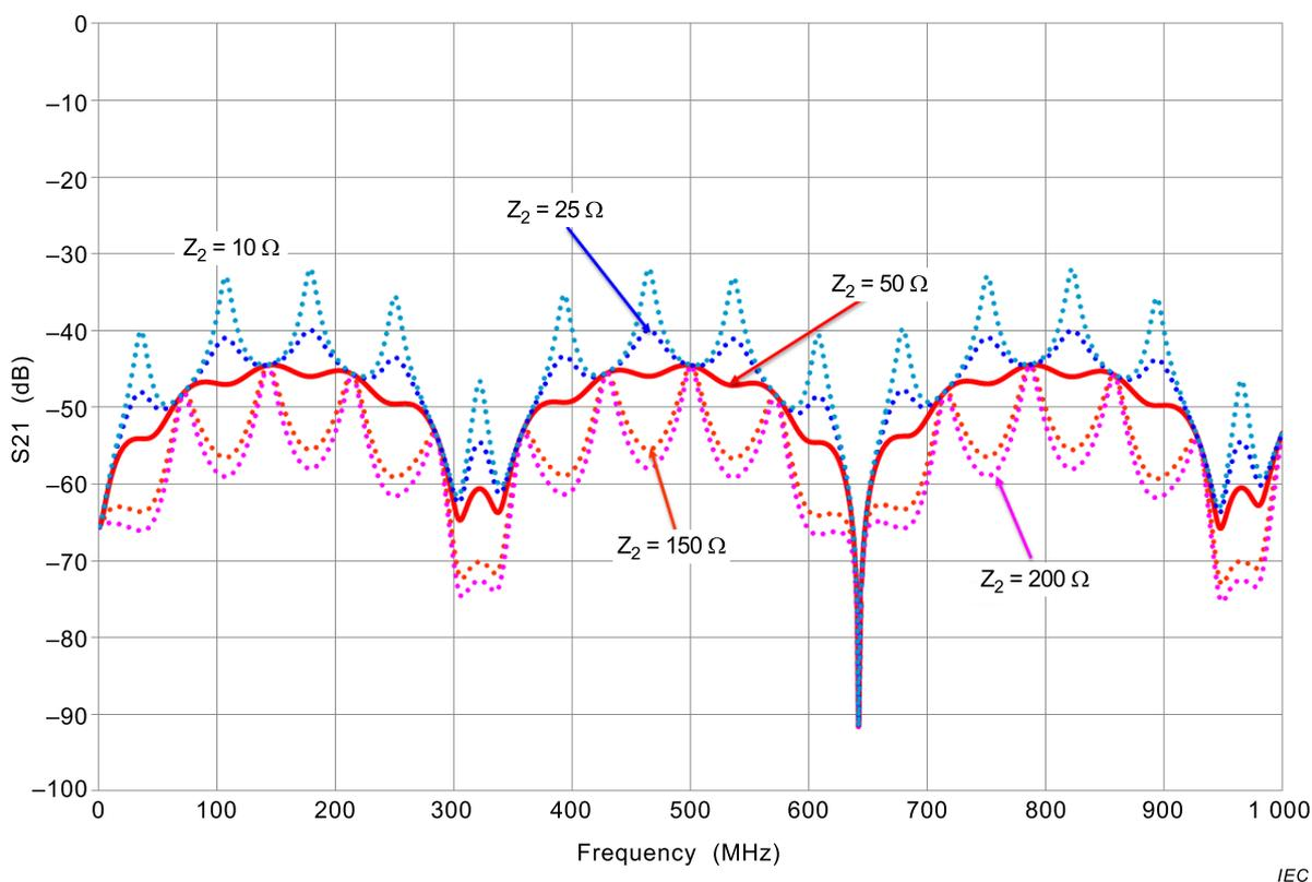
**Figure G.1 – Example of forward transfer scattering parameter  $S_{21}$  for different impedances in the outer circuit where the receiver input impedance is  $50\Omega$**
