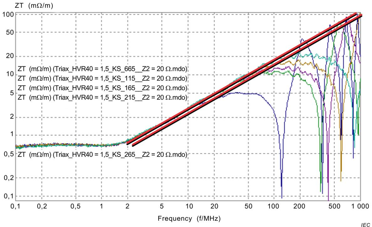
Figure F.5 – Compilation of transfer impedance test results with different shorting plane distances
