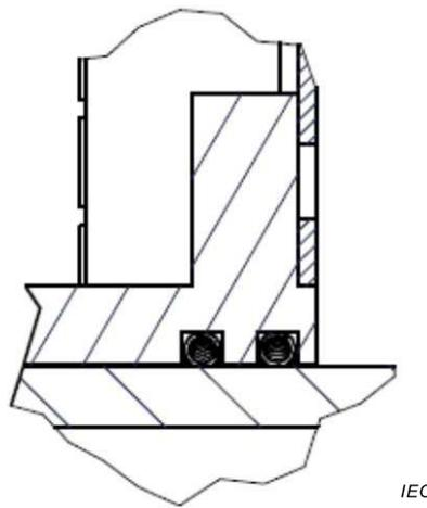
Figure F.4 – Detail G of figure F.2: contact between plane and tube-in-tube
