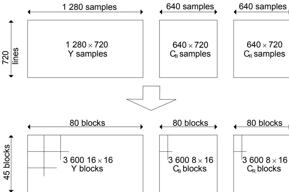
Figure 38 – 1280 × 720/P 4:2:2 YC<sub>B</sub>C<sub>R</sub> frame shuffle blocks
