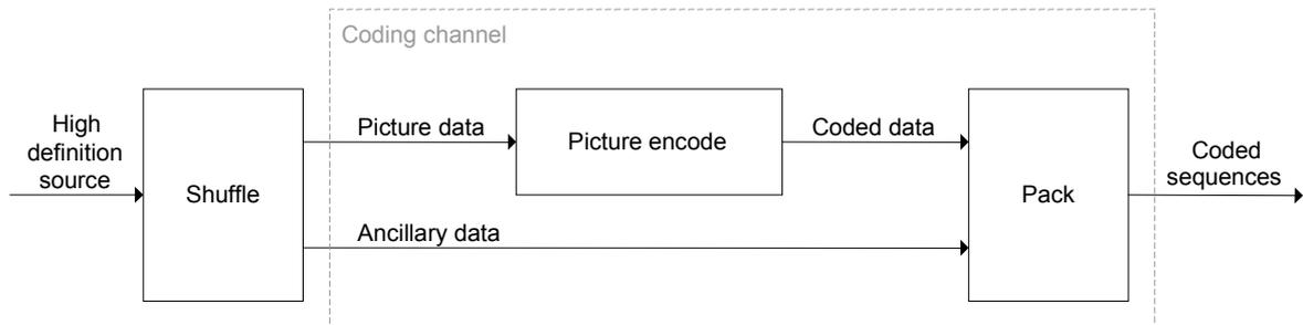
**Figure 32 – Type D-16 encoding, one coding channel**
