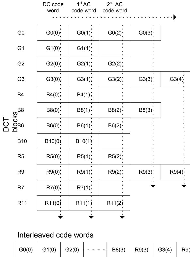
Figure 59 – 4:4:4 RGB DCT macro block interleaving example
