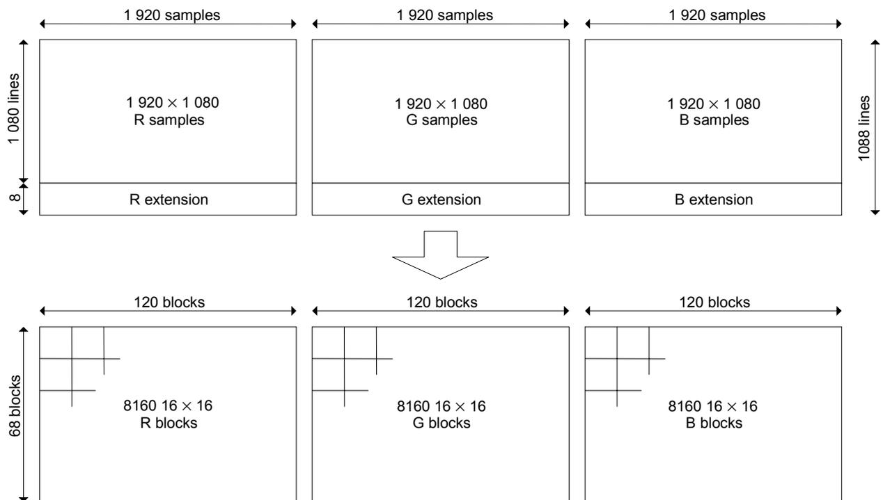
Figure 35 – 1920 × 1080/PsF 4:4:4 RGB shuffle blocks
