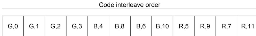
**Figure 58 – 4:4:4 DCT code interleave**
