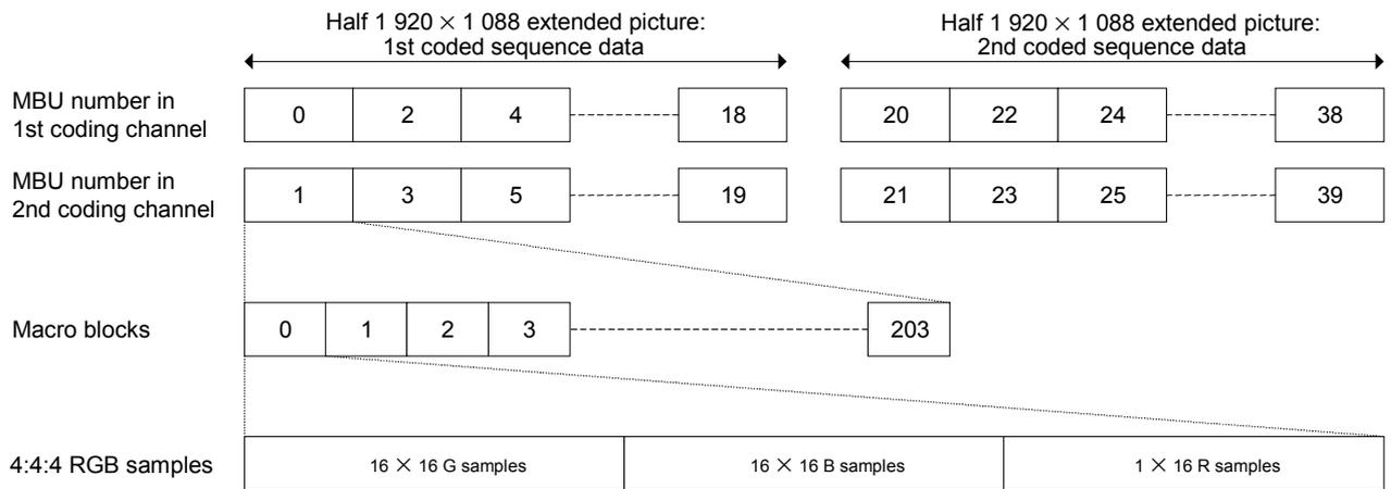
**Figure 45 – 1920 × 1080 4:4:4 RGB macro block unit number allocation**
