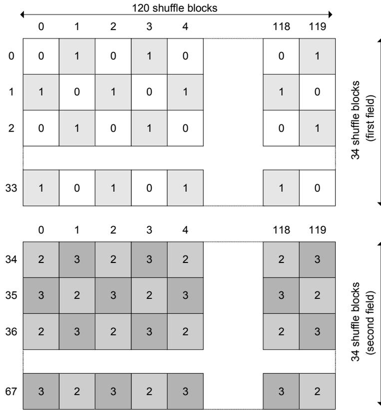
**Figure 41 – 1920 × 1080/I 4:2:2 YC<sub>B</sub>C<sub>R</sub> shuffle sets**
