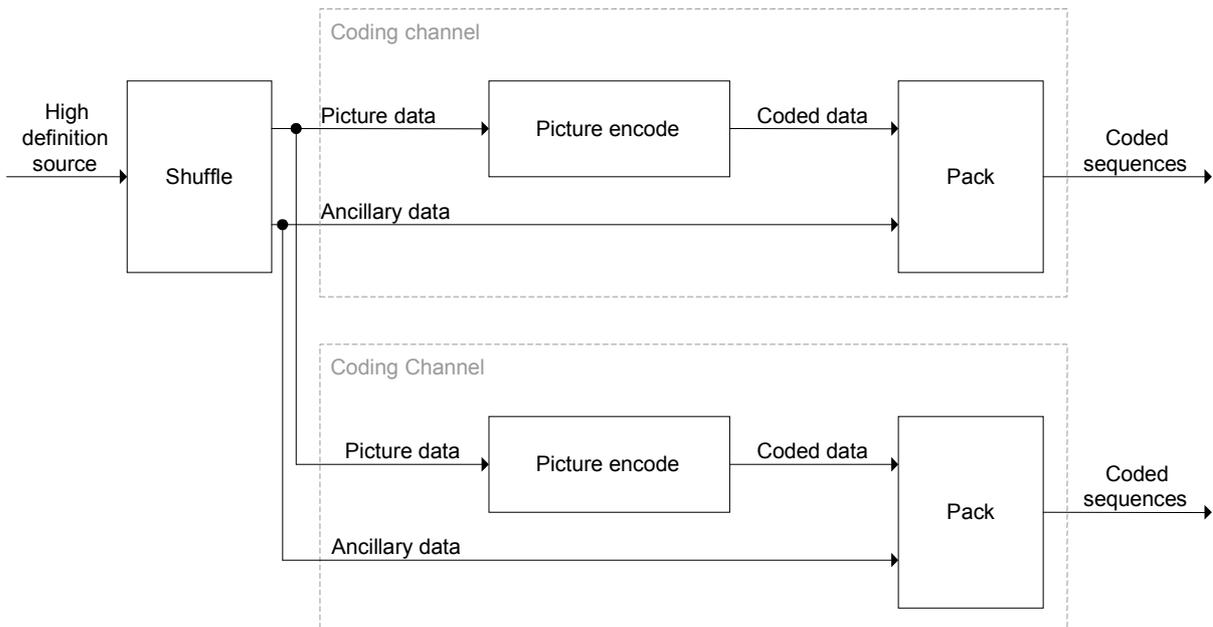
**Figure 33 – Type D-16 encoding, two coding channels**
