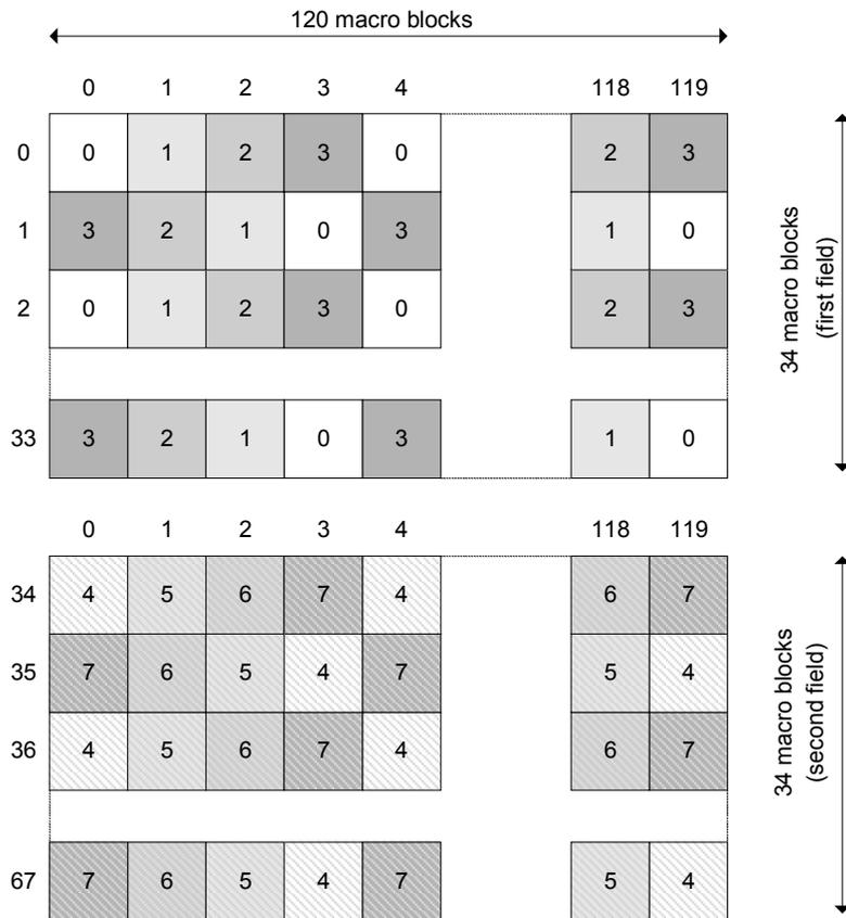
**Figure 42 – 1920 × 1080/I 4:4:4 RGB shuffle sets**
