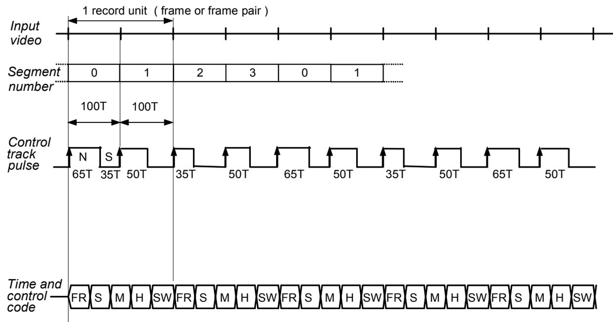
NOTE1 The following definitions are used in Figure 29: FR: frame; S: second; M: minute; H: hour; and SW: Sync Word.
