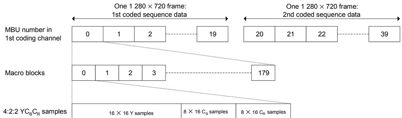
**Figure 46 – 1280×720 4:2:2 YC<sub>B</sub>C<sub>R</sub> macro block unit number allocation**
