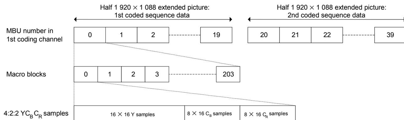
**Figure 44 – 1920x1080 4:2:2 YC<sub>B</sub>C<sub>R</sub> macro block unit number allocation**
