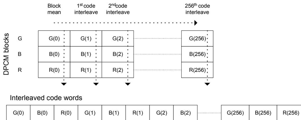
**Figure 63 – 4:4:4 RGB DPCM macro block interleaving example**
