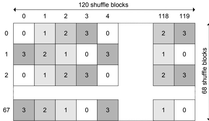
**Figure 39 – 1920 × 1080/PsF 4:2:2 YC<sub>B</sub>C<sub>R</sub> shuffle sets**
