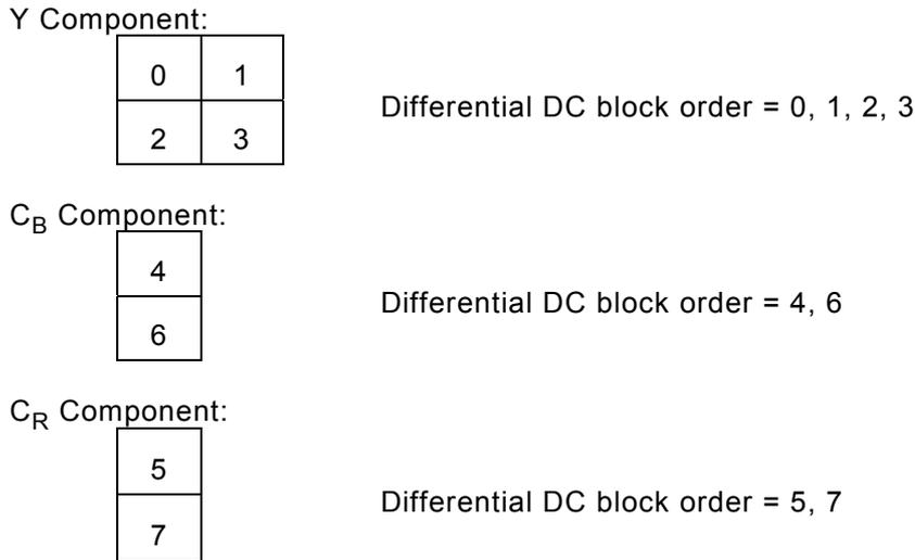
**Figure 54 – 4:2:2 YC<sub>B</sub>C<sub>R</sub> differential DC block order**
