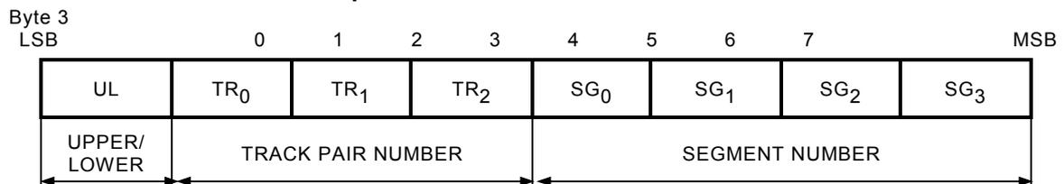
**Figure 76 – Sync block identification bytes**
