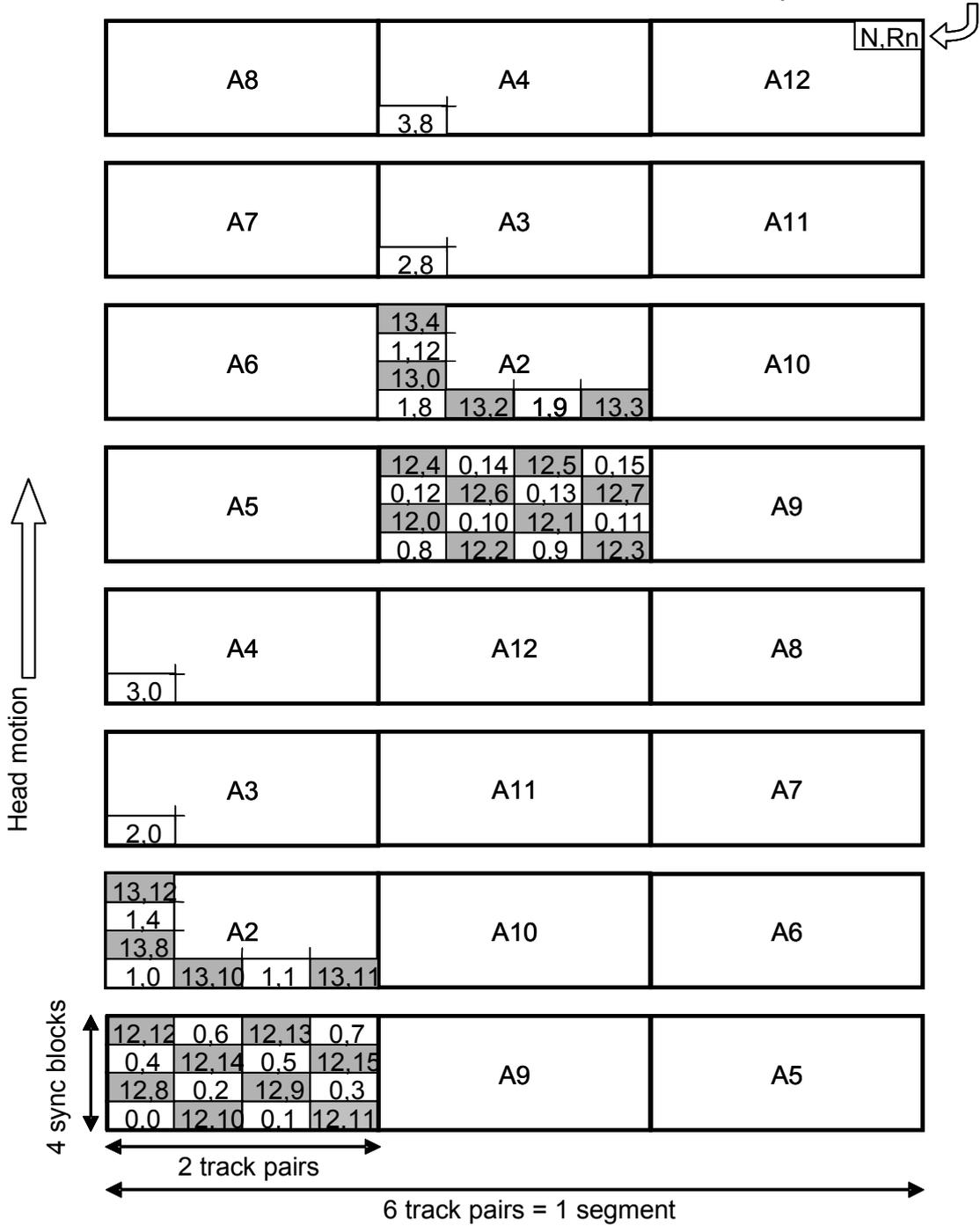
Figure 70 – Audio sync block alignments on helical tracks
