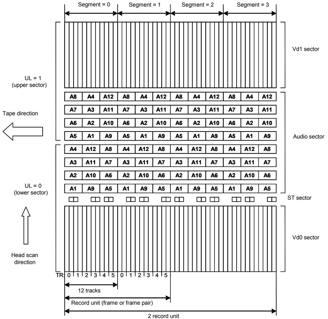
Figure 73 – Record unit, segment, channel and track pair counts
