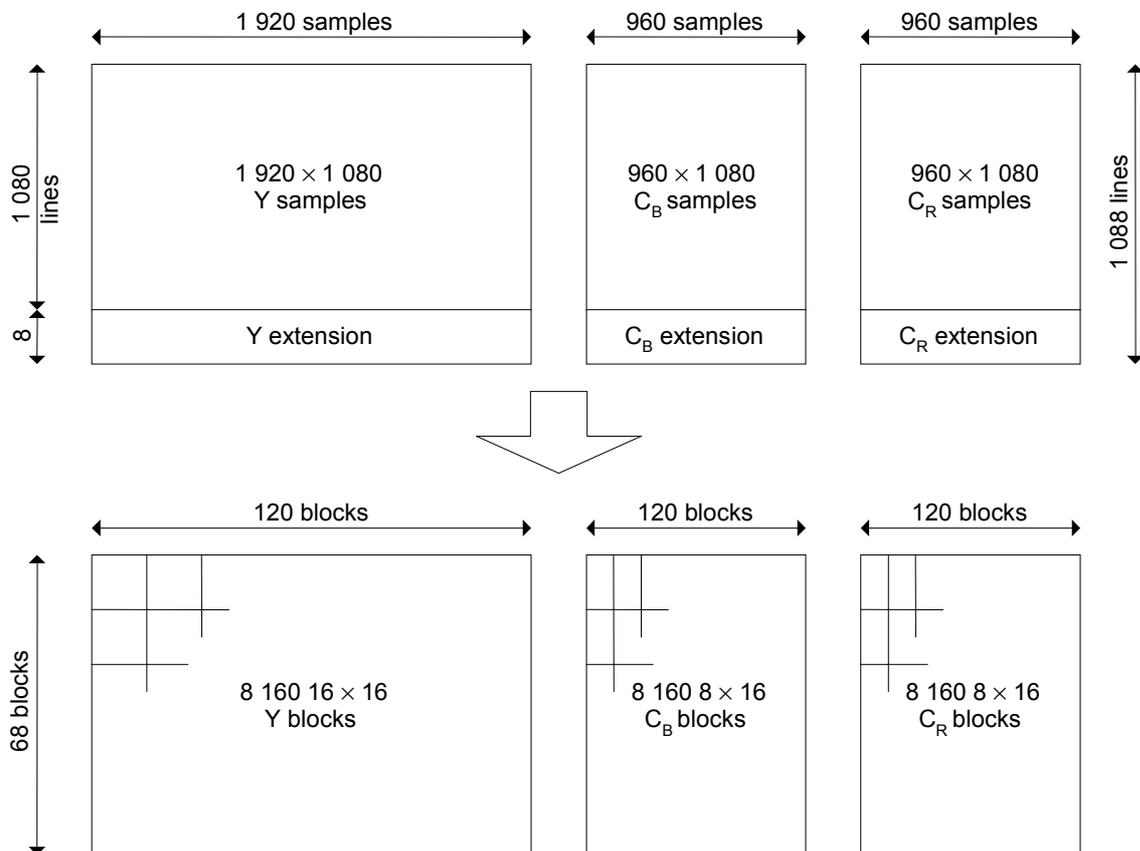
Figure 34 –  $1920 \times 1080$ /PsF 4:2:2  $Y C_B C_R$  shuffle blocks
