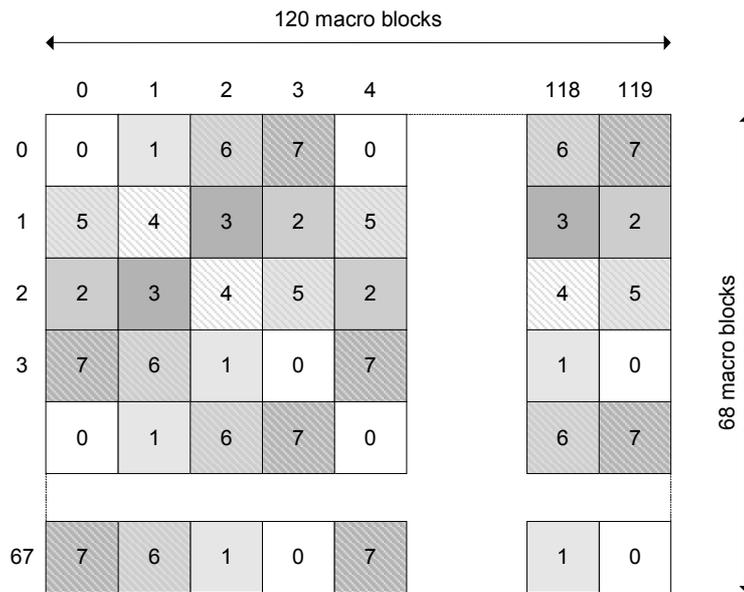
**Figure 40 – 1920 × 1080/PsF 4:4:4 RGB shuffle sets**
