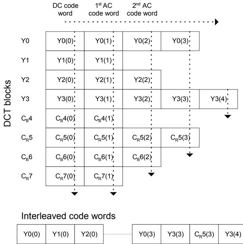
**Figure 57 – 4:2:2 Y<sub>C<sub>B</sub></sub>C<sub>R</sub> DCT macro block interleaving example**
