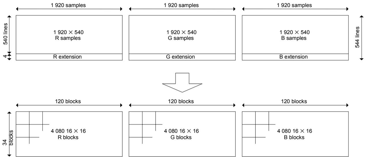
Figure 37 – 1920 × 540/l 4:4:4 RGB shuffle blocks
