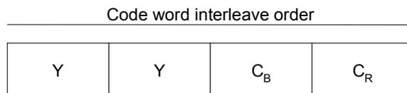
Figure 60 – 4:2:2 YC<sub>B</sub>C<sub>R</sub> DPCM code word interleave order
