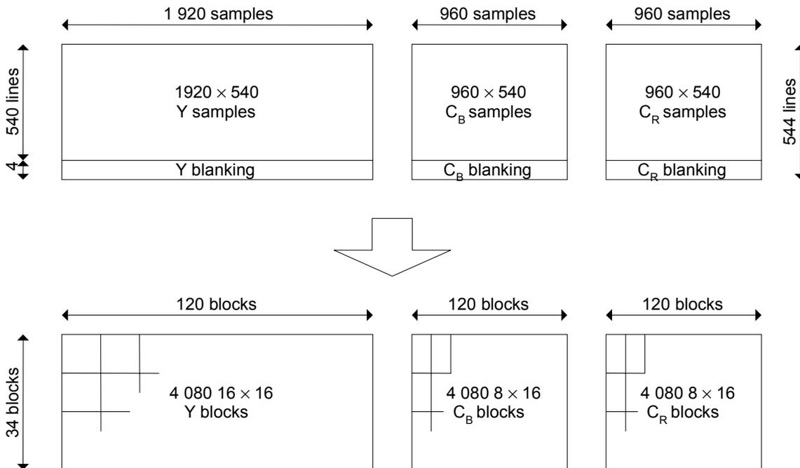
**Figure 36 –  $1920 \times 540/4:2:2 YC_B C_R$  shuffle blocks**
