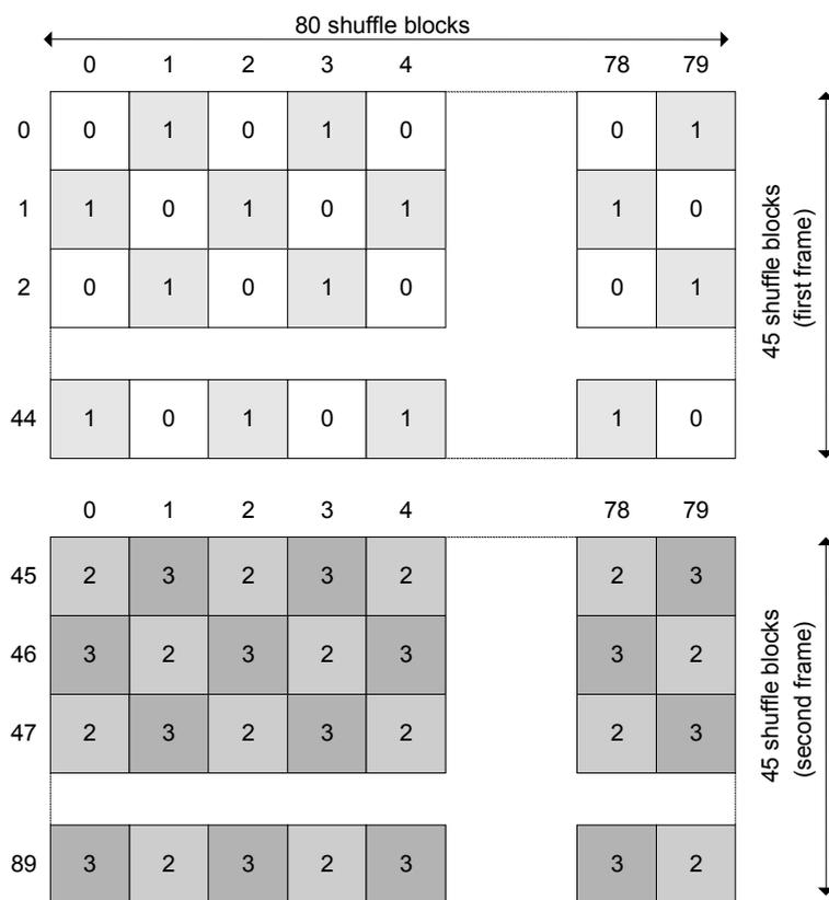
**Figure 43 – 1280 × 720/P 4:2:2 YC<sub>B</sub>C<sub>R</sub> shuffle sets**
