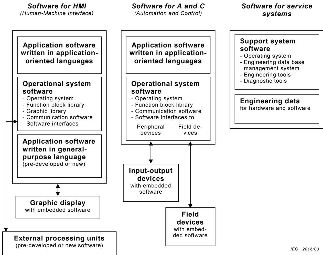
Figure 1 – Typical software parts in computer-based I&C systems
