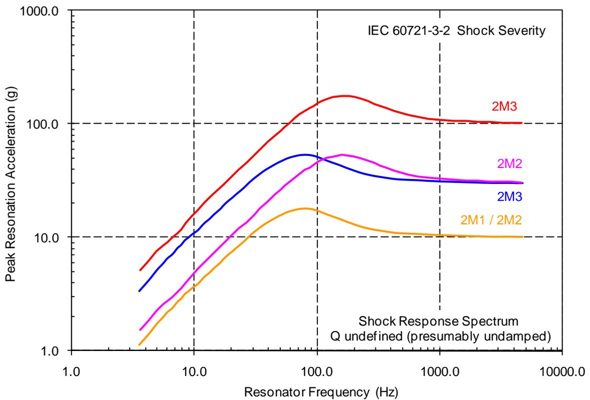
Figure 32 – IEC 60721-3-2:1997 – Non-stationary vibration including shock
