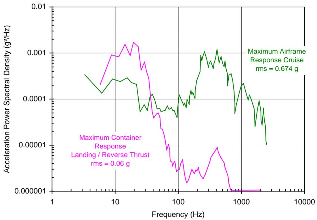
**Figure 21 – VC10 measurements – Overlaid worst case spectra**
