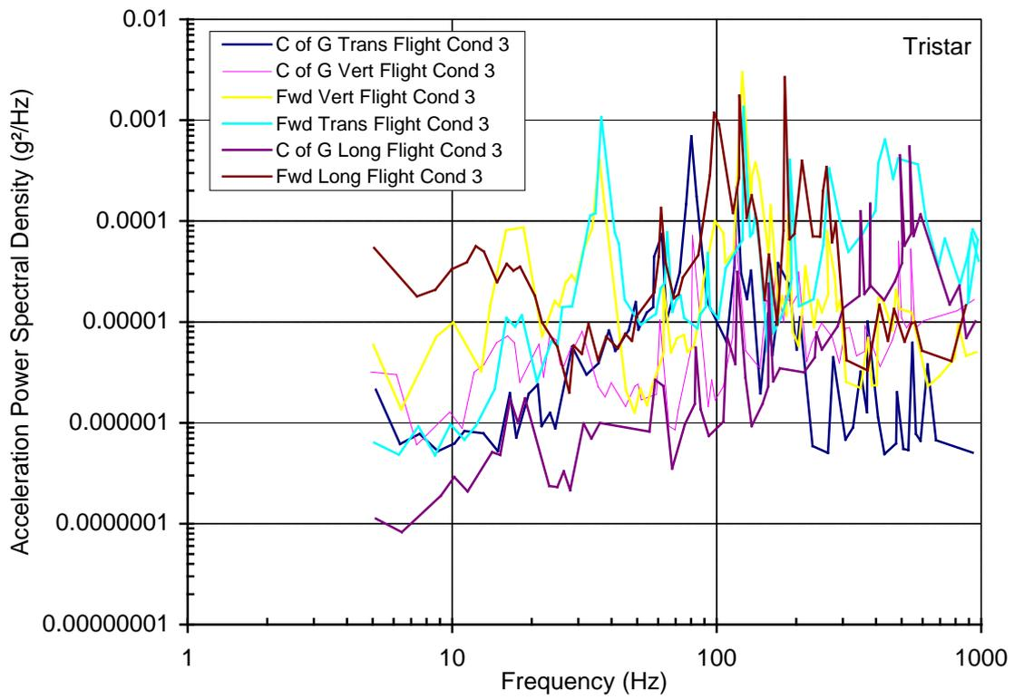
Figure 4 – Tristar vibration measurements – Low altitude climb
