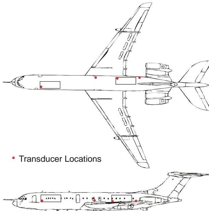
**Figure 16 – Schematic of VC10 aircraft**
