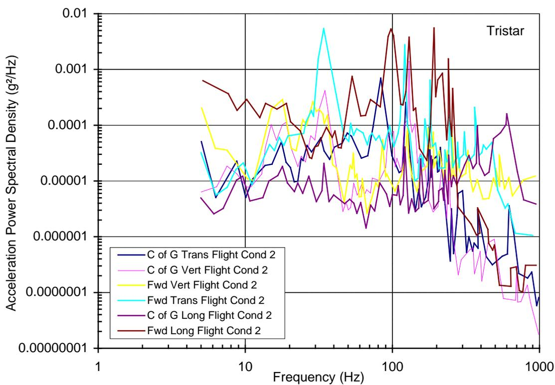
Figure 3 – Tristar vibration measurements – Take-off, power and roll
