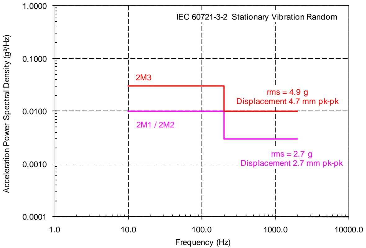
Figure 31 – IEC 60721-3-2:1997 – Stationary vibration random
