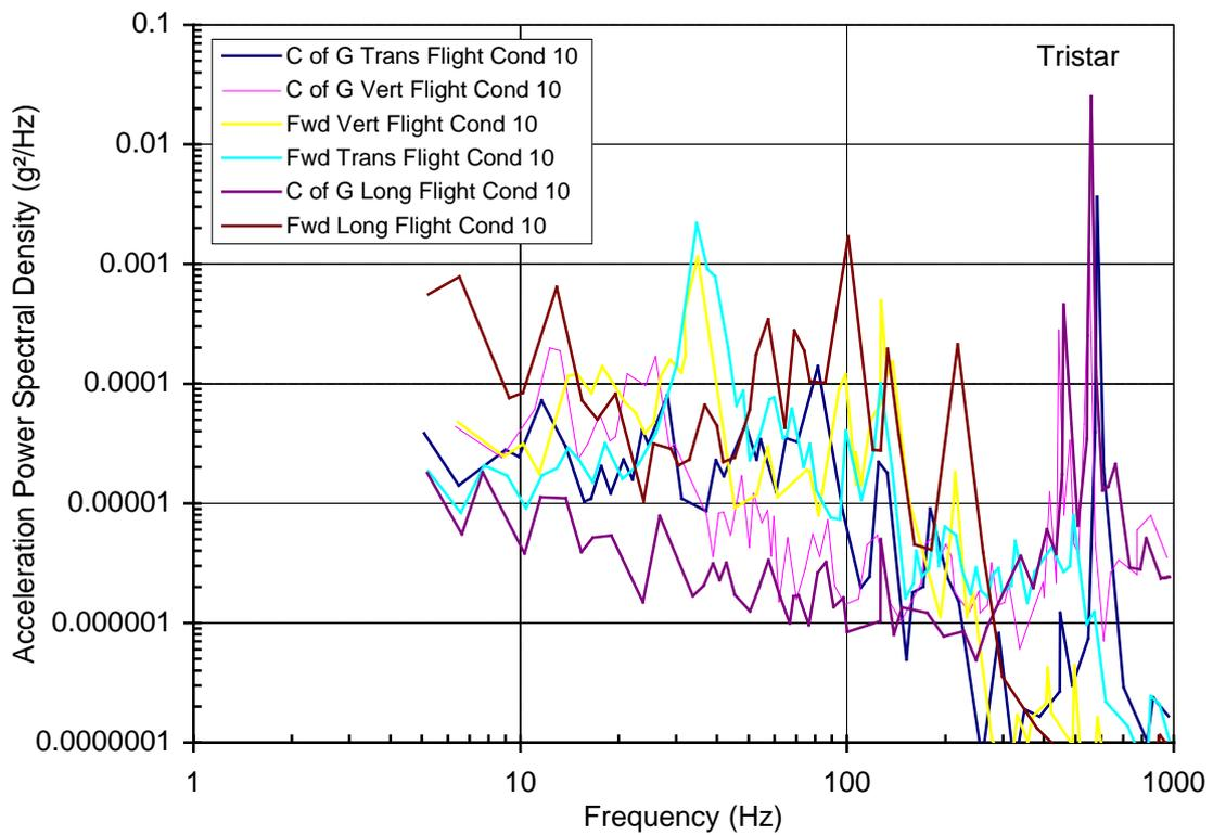
Figure 7 – Tristar vibration measurements – Low altitude decent
