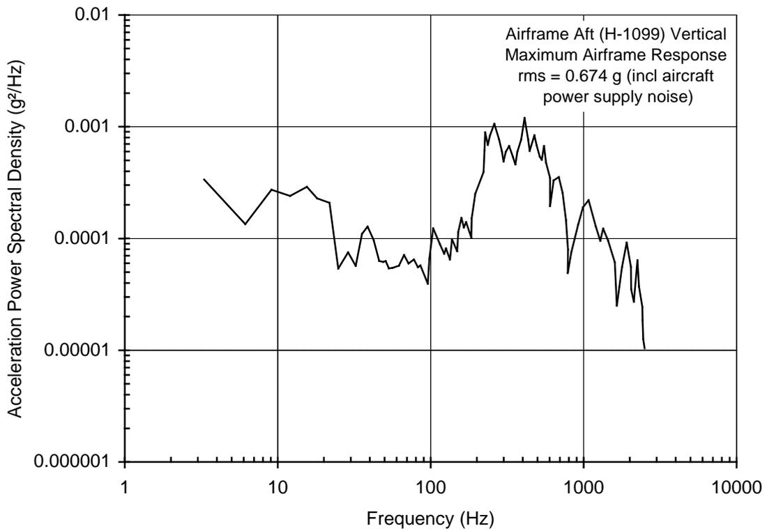
Figure 18 – VC10 vibration measurements – Maximum airframe severity
