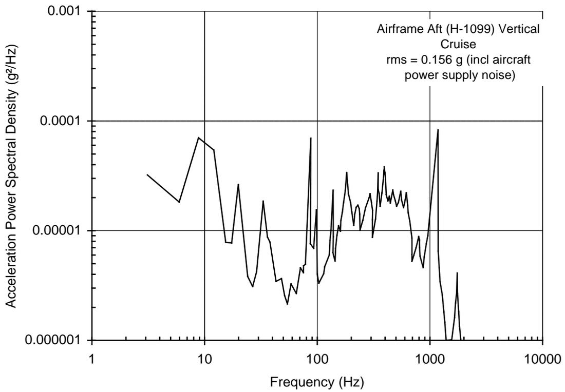
Figure 17 – VC10 vibration measurements – Cruise
