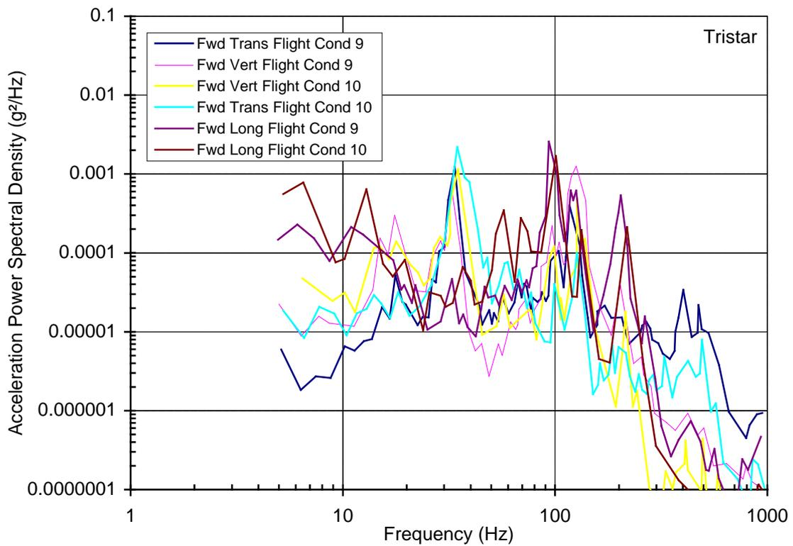
Figure 13 – Tristar vibration measurements – Forward landing
