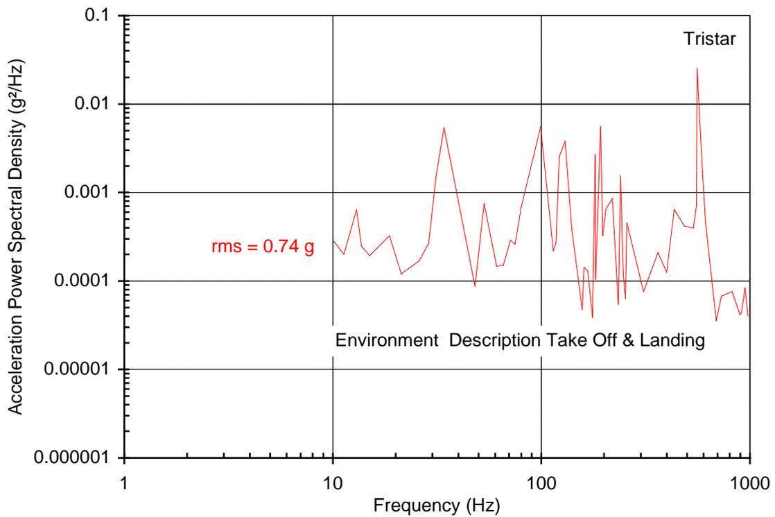
Figure 15 – Tristar vibration measurements – Take-off/landing environment
