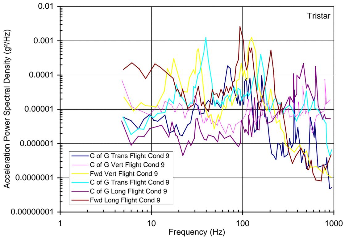
Figure 6 – Tristar vibration measurements – Landing
