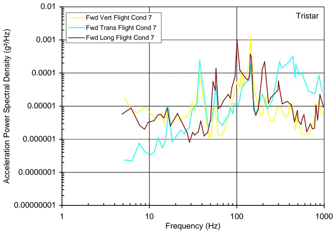
Figure 11 – Tristar vibration measurements – Forward cruise
