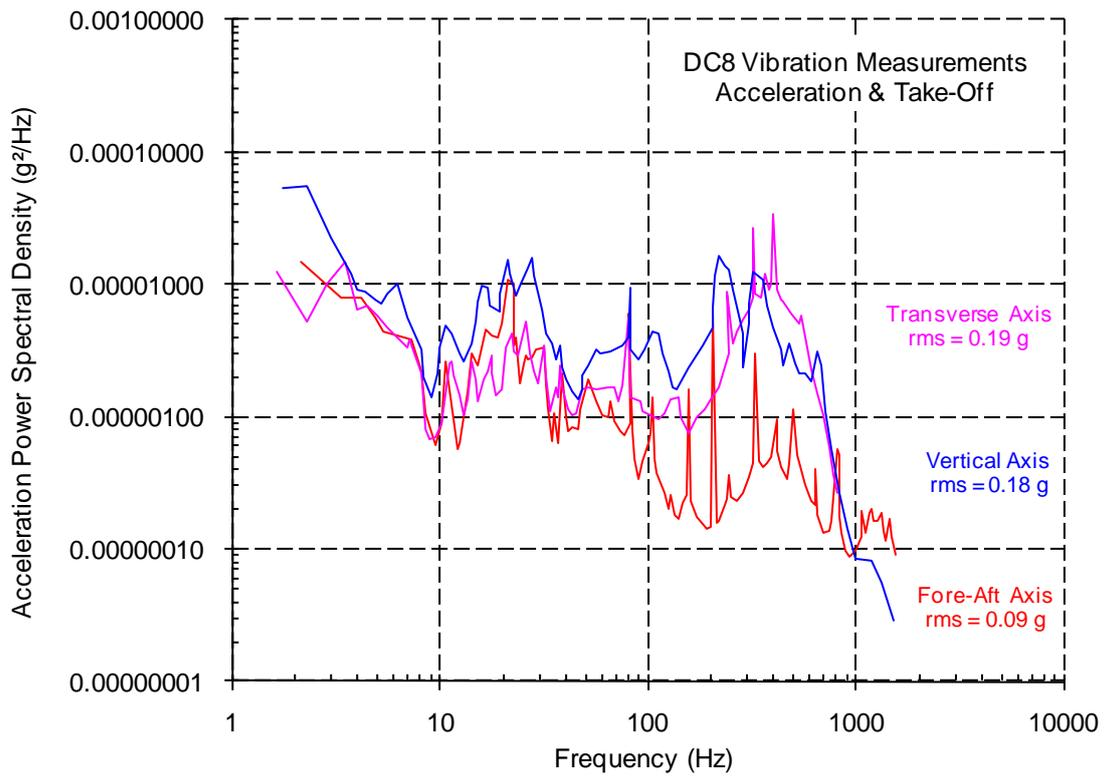
Figure 25 – DC8 vibration measurements acceleration and take-off
