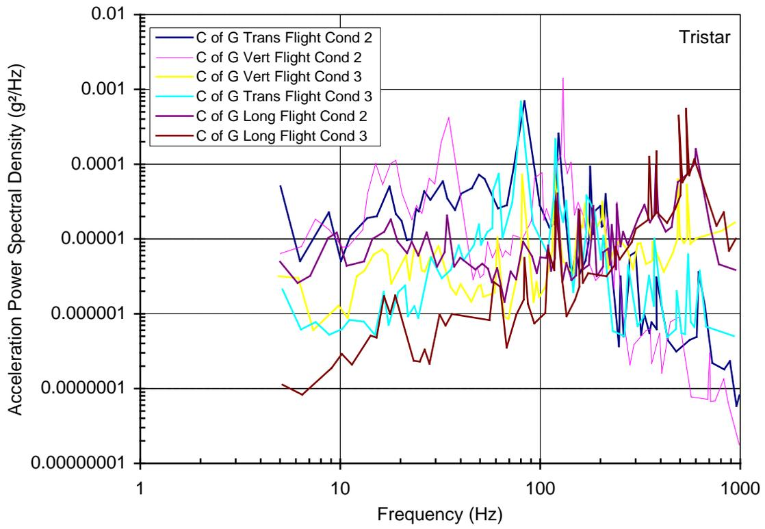
**Figure 8 – Tristar vibration measurements – C of G take-off/climb**
