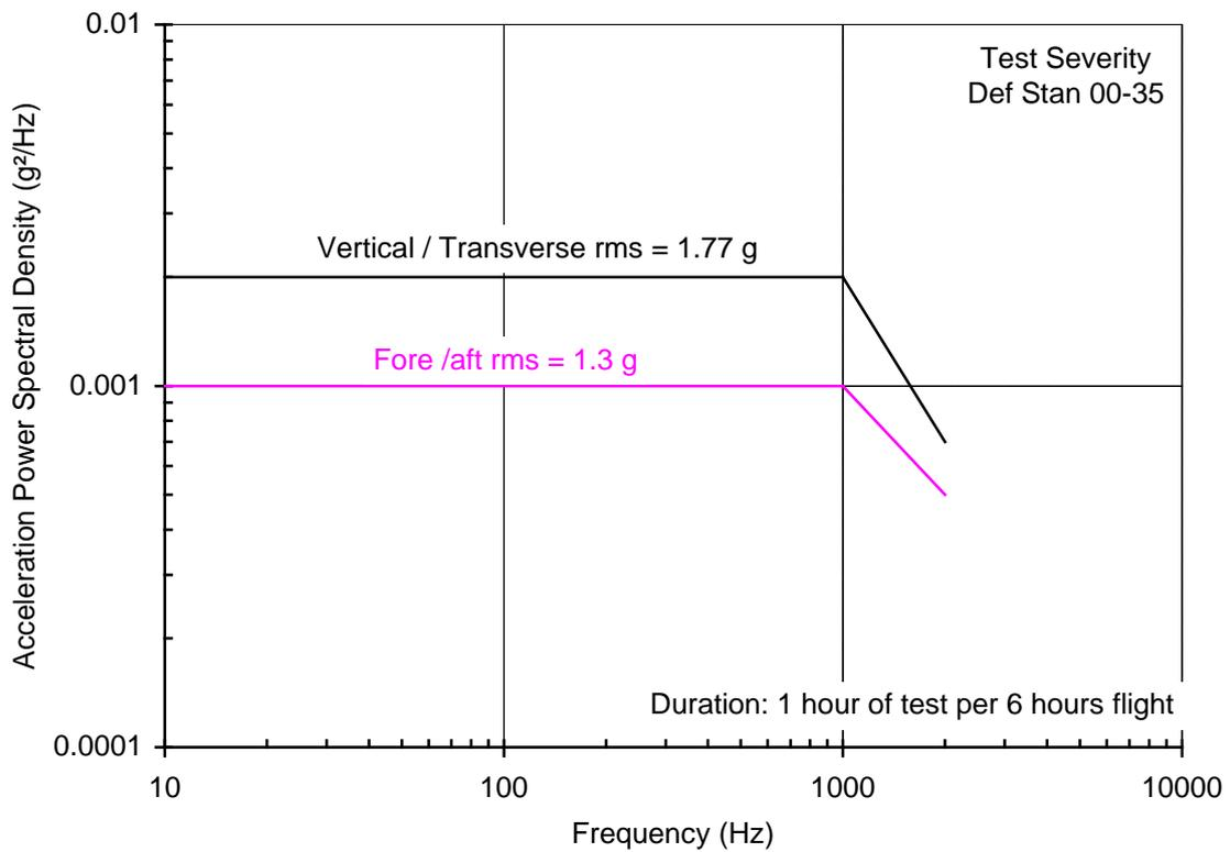
Figure 36 – Test severity – Def Stan 00-35, issues 3 and 4
