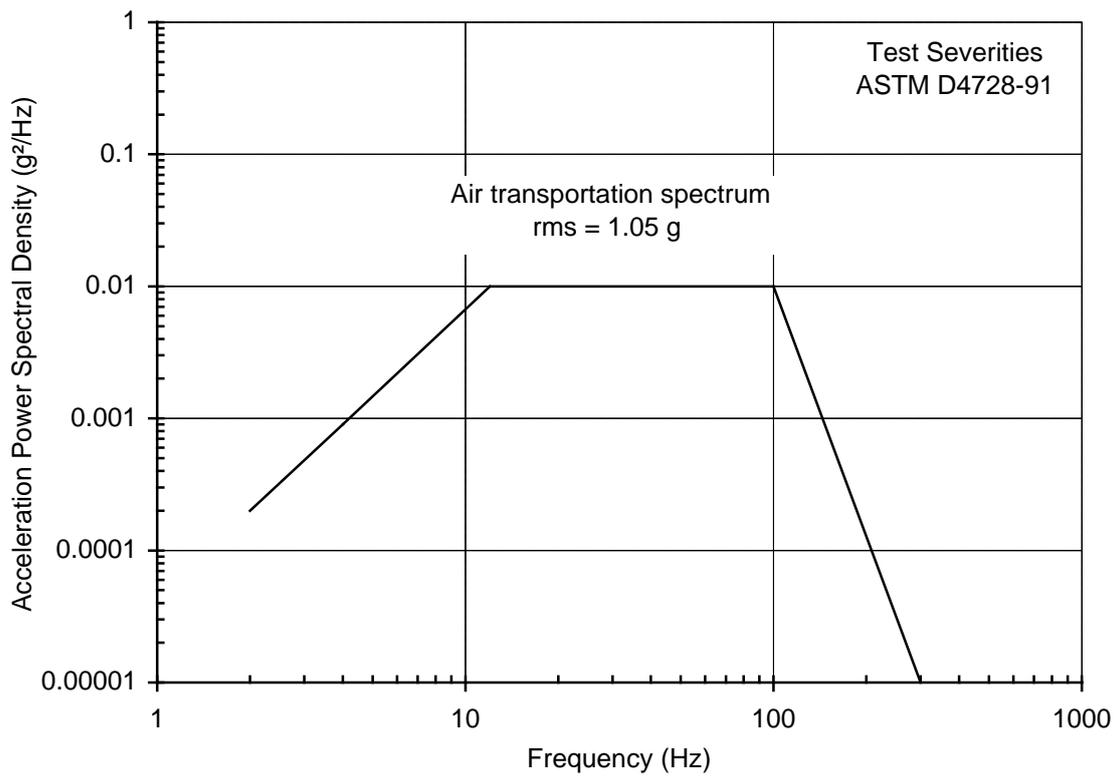
Figure 33 – Test severities – ASTM D 4728-91
