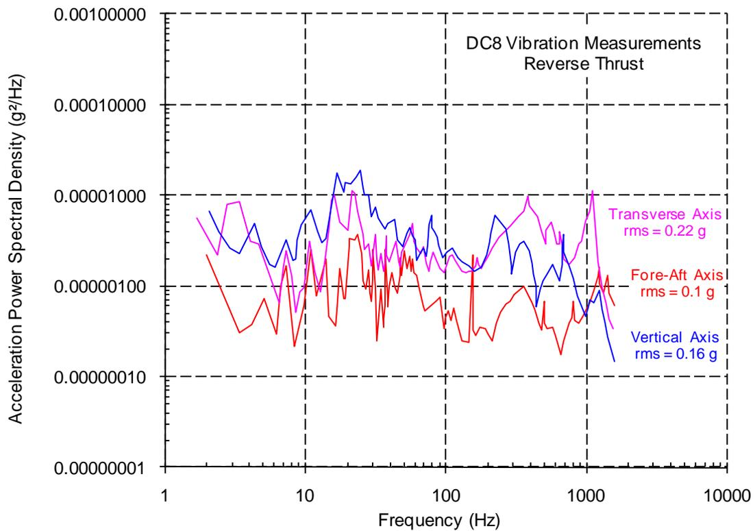
**Figure 24 – DC8 vibration measurements reverse thrust**
