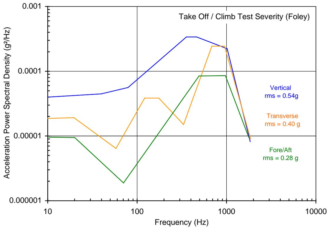
**Figure 29 – Foley test severity for take-off/landing**
