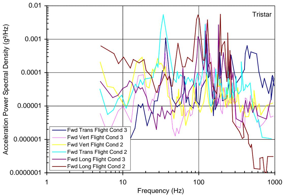
**Figure 9 – Tristar vibration measurements – Forward take-off/climb**
