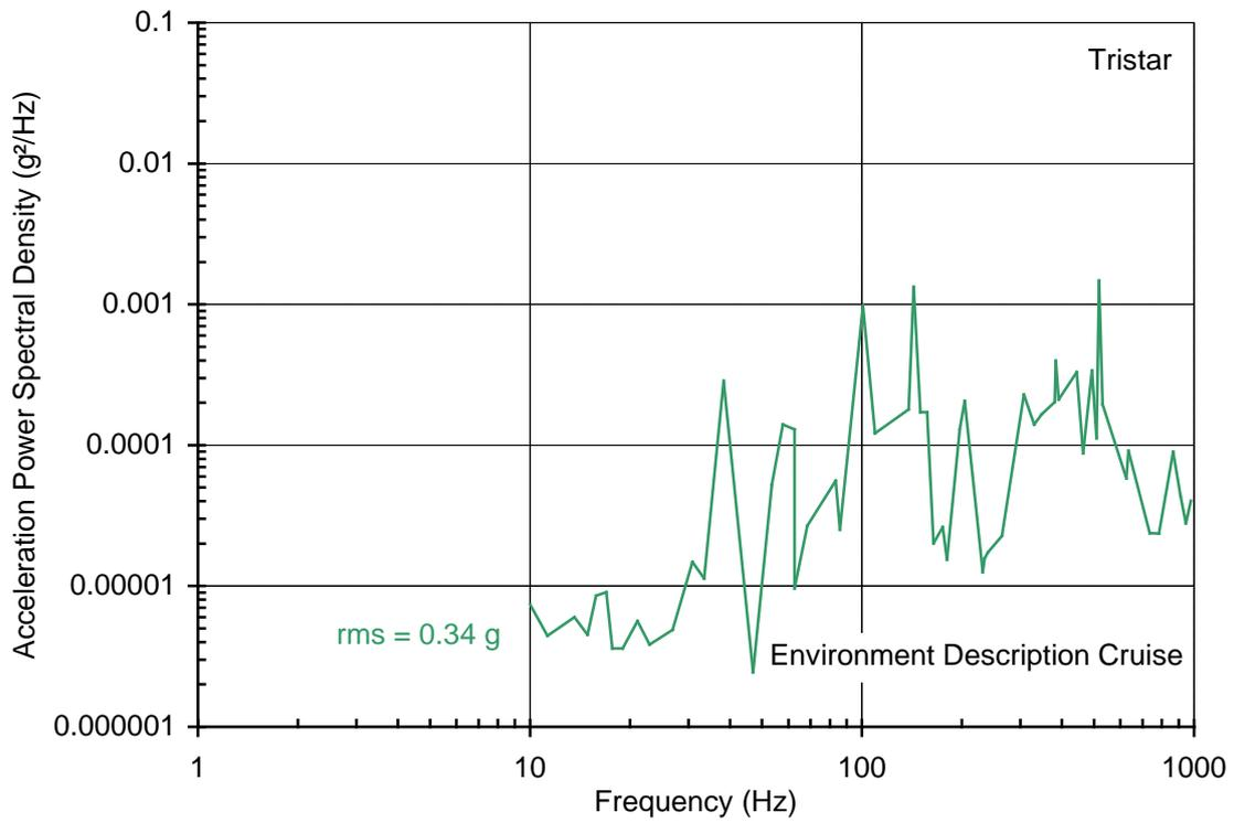
Figure 14 – Tristar vibration measurements – Cruise environment
