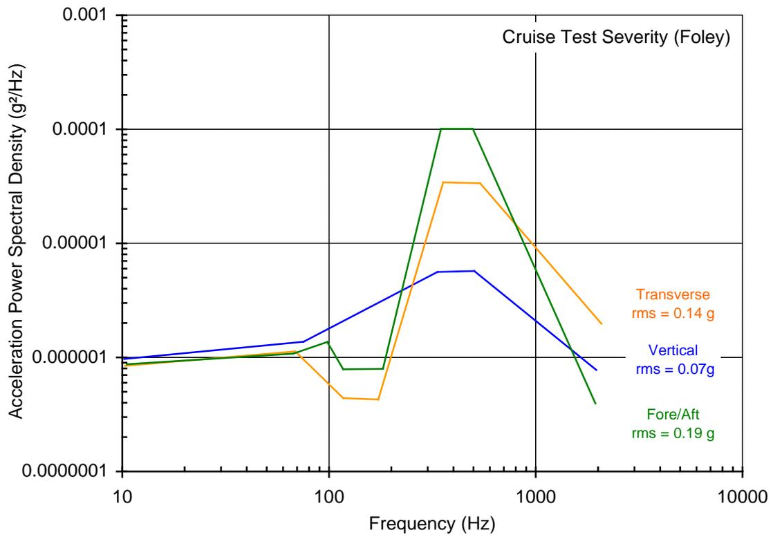
**Figure 30 – Foley test severity for cruise**
