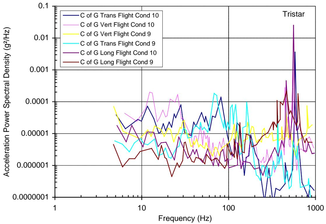
Figure 12 – Tristar vibration measurements – Centre of gravity landing
