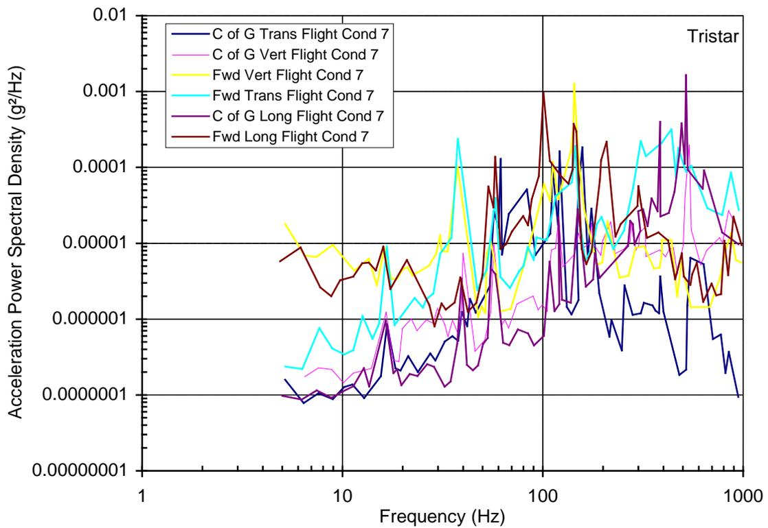
Figure 5 – Tristar vibration measurements – High altitude cruise
