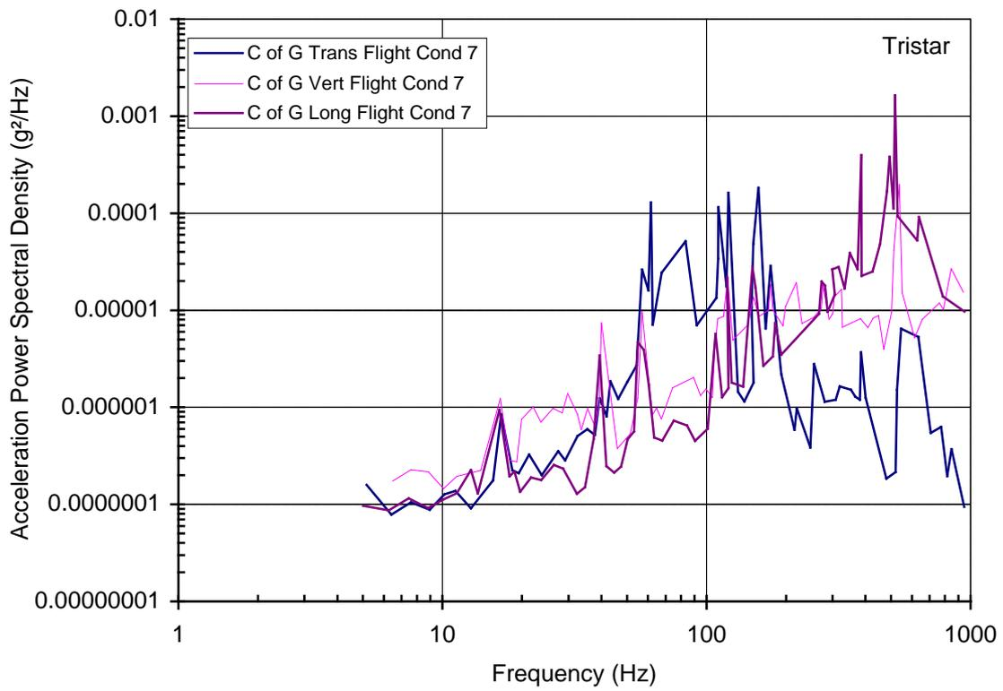
Figure 10 – Tristar vibration measurements – Centre of gravity cruise
