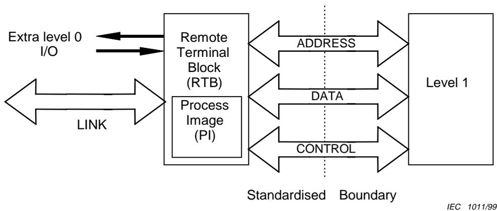
**Figure 14 – RTB interface to level 1 equipment**
