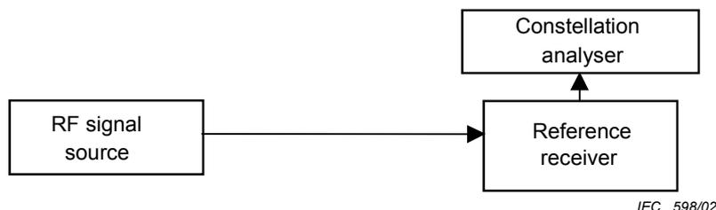
**Figure 11 – Test set-up for MER measurement**
