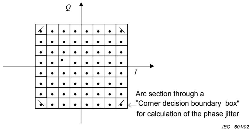
Figure 14 – Example of constellation diagram for a 64QAM modulation format where are shown the "corner decision boundary boxes" for the phase jitter
