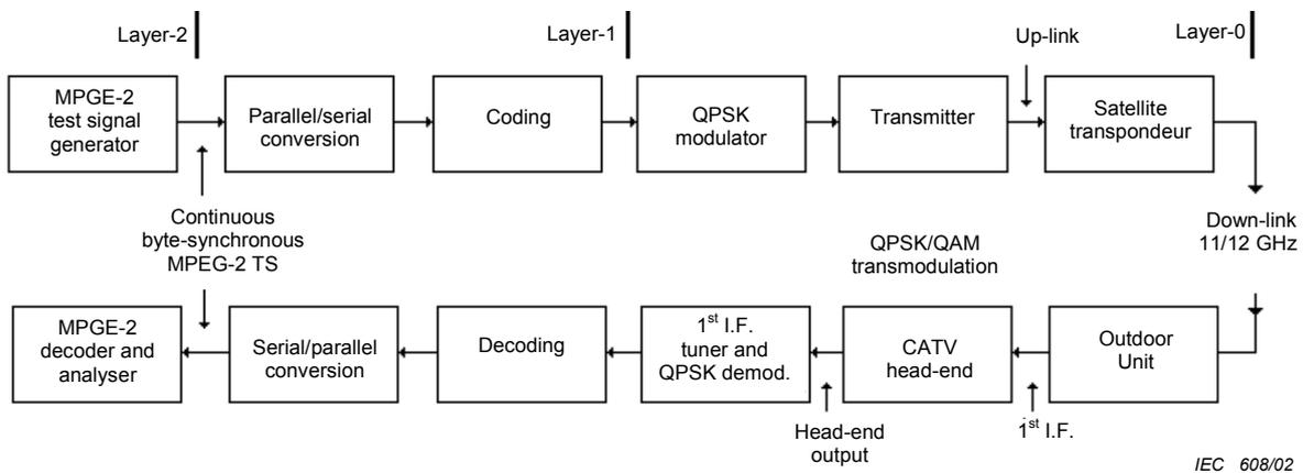
**Figure 21 – Measurement set-up for the evaluation of the MPEG-2 transport stream parameters for a communication link that feeds a CATV system using a satellite transponder and a down link in the 11/12 GHz band**
