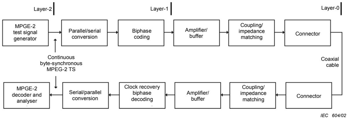
**Figure 17 – Measurement set-up for the evaluation of the MPEG-2 transport stream parameters for a communication link using a coaxial cable and synchronous serial transmission (SSI type)**
