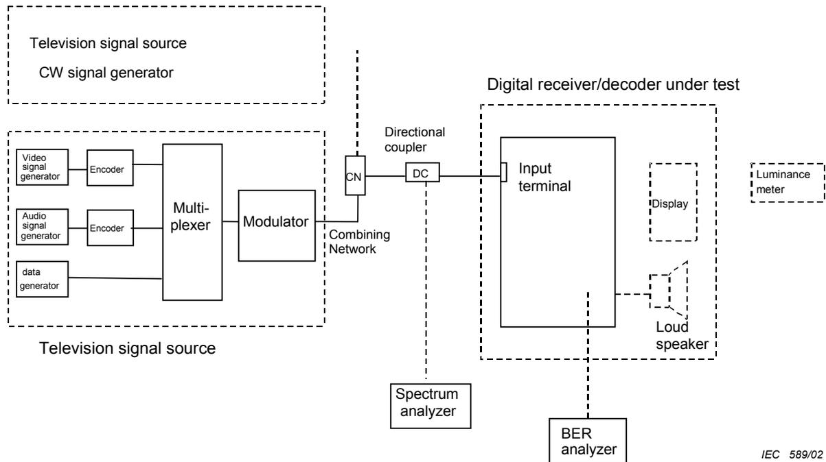
Figure 2 – Measuring set-up
