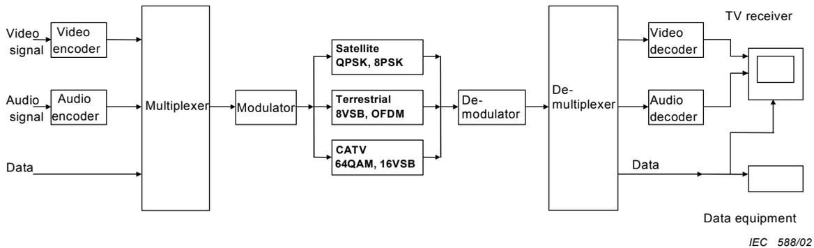
Figure 1 – Conceptual configuration of a digital broadcasting system
