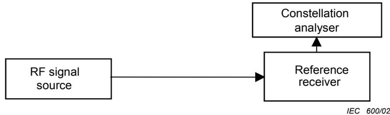
Figure 13 – Test set-up for phase jitter measurement
