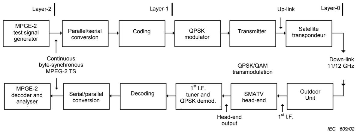
**Figure 22 – Measurement set-up for the evaluation of the MPEG-2 transport stream parameters for a communication link that feeds a SMATV system using a satellite transponder and a down link in the 11/12 GHz band**
