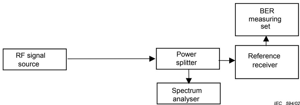
**Figure 7 – Test set-up for BER measurement**
