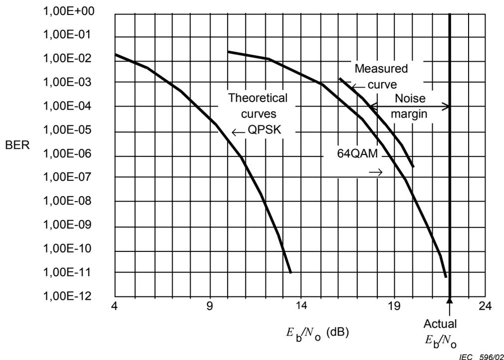
**Figure 9 – Example of BER measurement versus  $E_b/N_o$**
