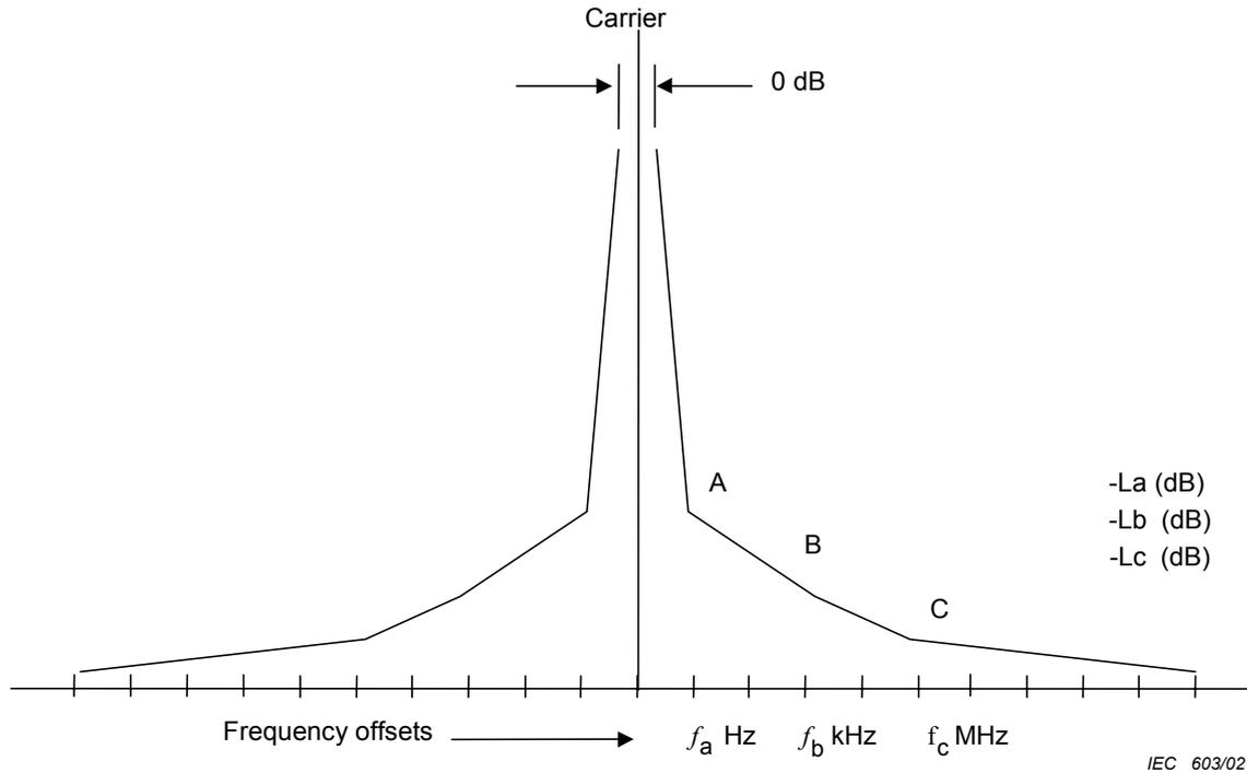
**Figure 16 – Possible mask for CPE measurements – the points A, B and C to be defined**
