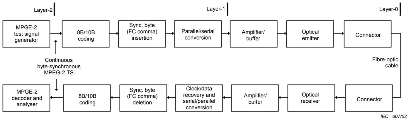
**Figure 20 – Measurement set-up for the evaluation of the MPEG-2 transport stream parameters for a communication link using a fibre-optic cable and asynchronous serial transmission (ASI type)**
