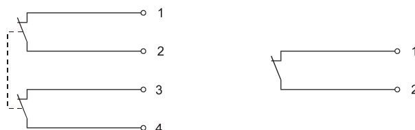
Figure A.7 – Connection of mechanical switches
