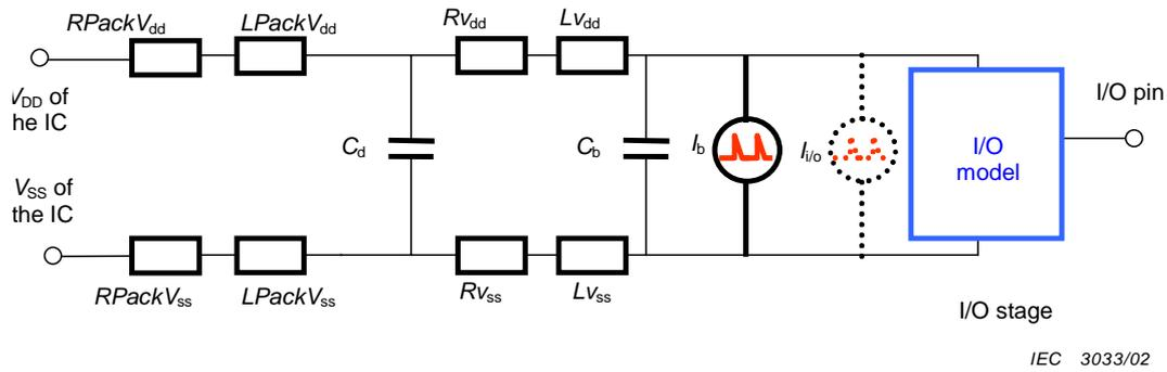
Figure 7 – Coupling between core and I/Os
