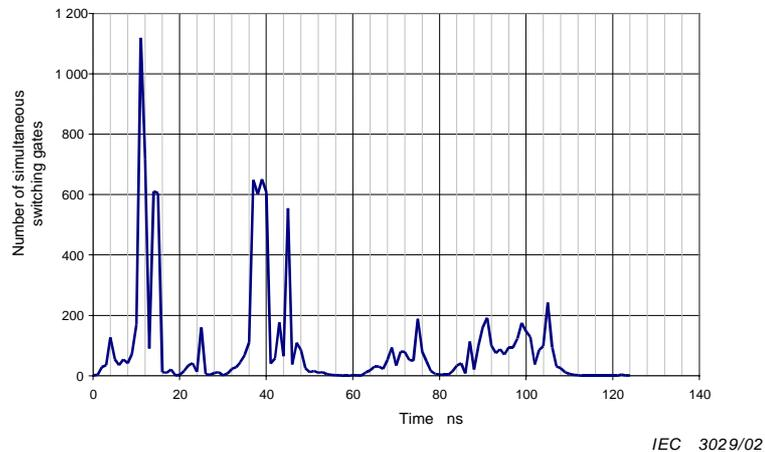
Figure 3 – Number of switching gates versus time
