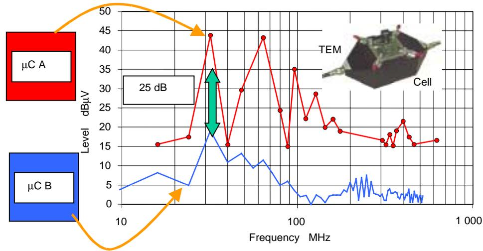
Figure 9 – IC direct emissions measured in TEM cell
