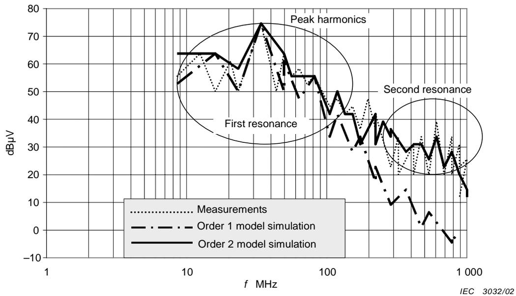
Figure 6 – Comparison between simulation and measurements (IEC 61967-4, 1  $\Omega$  method)
