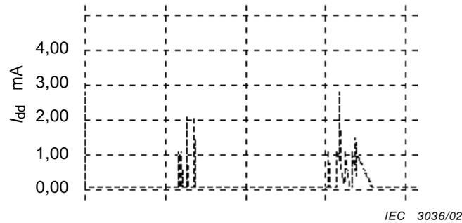
Figure 10 – Current source definition as a PWL description versus time
