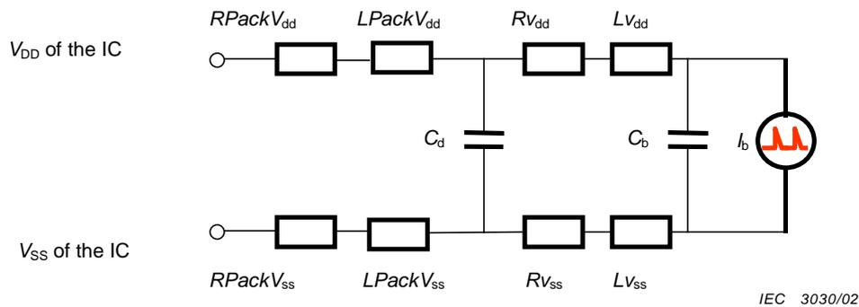
Figure 4 – Model of the IC supply lines
