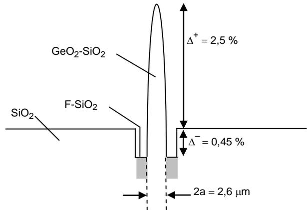
**Figure A.3b – Double cladding type**
