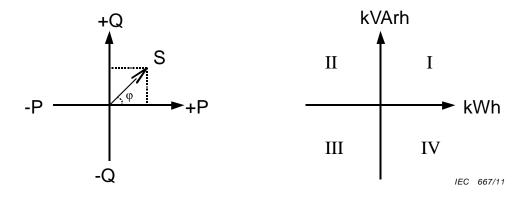
NOTE 1 Power is often computed as the vector S=P+jQ, where reactive power (Q, in VAr units) is plotted on the ordinate axis, and real power (P, in Watts) is plotted on the abscissa. Four-quadrant metering is the extension of
