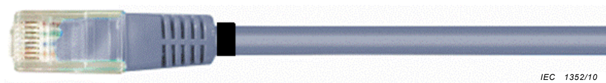
Figure 4 – Initial marking of the cable sheath
