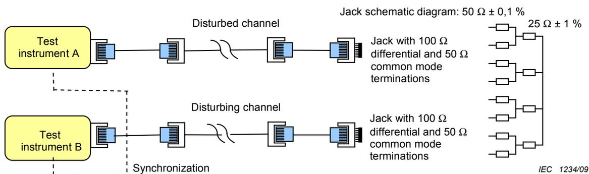
**Figure 19 – Schematic diagram to measure channel ANEXT loss**
