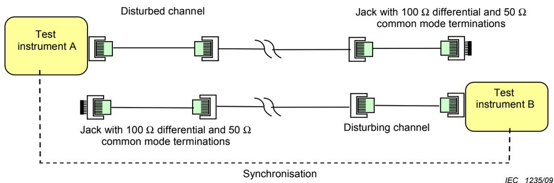
**Figure 20 – AFEXT loss measurement test configuration**
