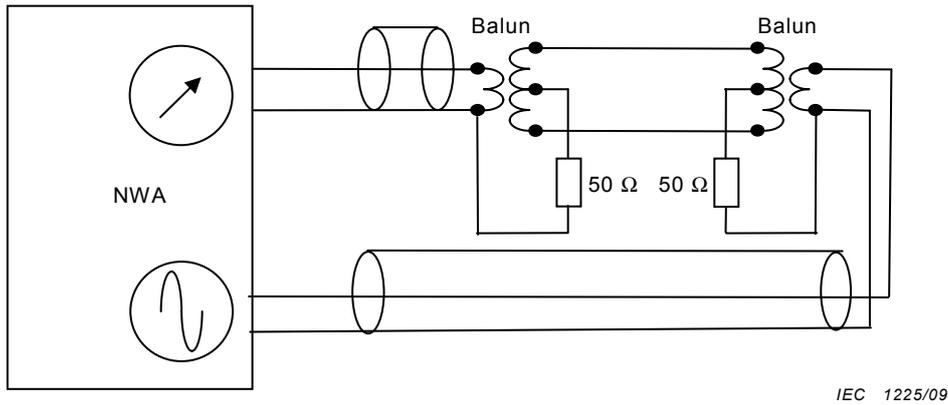
Figure 13 – Back-to-back balun differential mode insertion loss measurement
