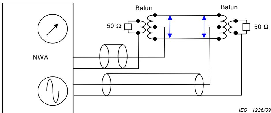
Figure 14 – Back-to-back balun common mode insertion loss measurement
