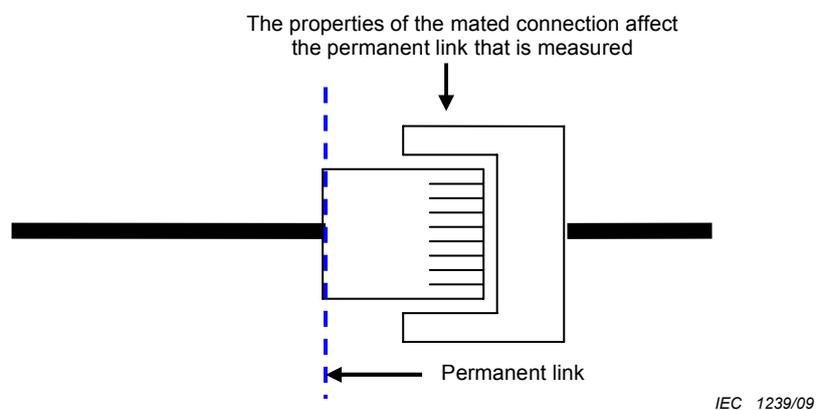
**Figure A.1 – Source of variability during link testing**
