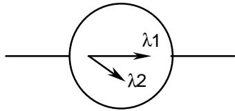
NOTE – Normally open represents a switch that in the unactuated condition blocks a wavelength of light  $\lambda_2$  and allows a wavelength of light  $\lambda_1$  to travel down the fibre. Actuating the switch will allow a wavelength of light  $\lambda_2$  to travel down the fibre and block a wavelength of light  $\lambda_1$ .
