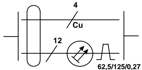
NOTE – An example of a composite cable containing both copper conductors and optical fibres with supplementary information is shown. This specific example shows the composite cable containing four copper conductors along with 12 multimode graded-index optical fibres, each with a core diameter of 62.5 µm and cladding diameter of 125 µm and NA of 0.27.
