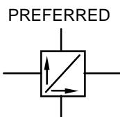
NOTE – This symbol is for a bulk optic cube beamsplitter. Since this device is reversible, the arrows can be reversed to indicate a bulk optic combiner or multiplexer.
