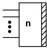
NOTE – In a star branching device of this type, each port is bidirectional and may be used simultaneously as an input and an output. Each port feeds every other port.
