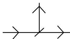
NOTE – A 1 to 2 splitter is shown. A 1 to 2 splitter is also known as a passive tap.
