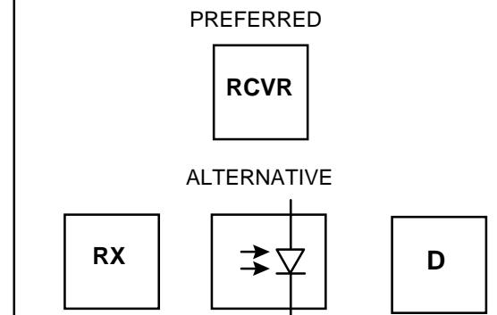
**3.28.2 Guided light unconnectorized (pigtailed) receiver**
