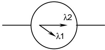
NOTE – Normally closed represents a switch that in the unactuated condition blocks a wavelength of light  $\lambda_1$  and allows a wavelength of light  $\lambda_2$  to travel down the fibre. Actuating the switch will allow a wavelength of light  $\lambda_1$  to travel down the fibre and block a wavelength of light  $\lambda_2$ .
