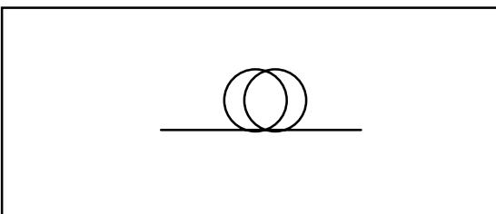
**3.29 Receptacle, with optical source**
