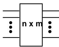
NOTE – An  $n \times m$  star branching device is shown.  $n$  and  $m$  can be specified. A passive version of this device is sometimes referred to as an optical combiner.
