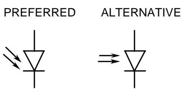
NOTE – Also known as a PIN detector. See light emitting diode for a pigtailed example.
