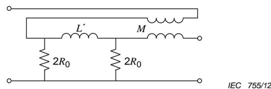
**Figure 48 – Equivalent circuit for a compensated shunt**
