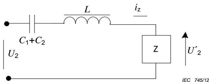
**Figure 22 – Simplified CVT Thevenin equivalent circuit at power frequency**
