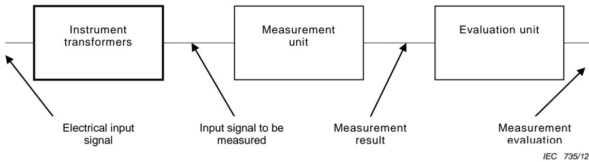
**Figure 1 – Measurement chain (From h)<sup>1</sup>, modified)**
