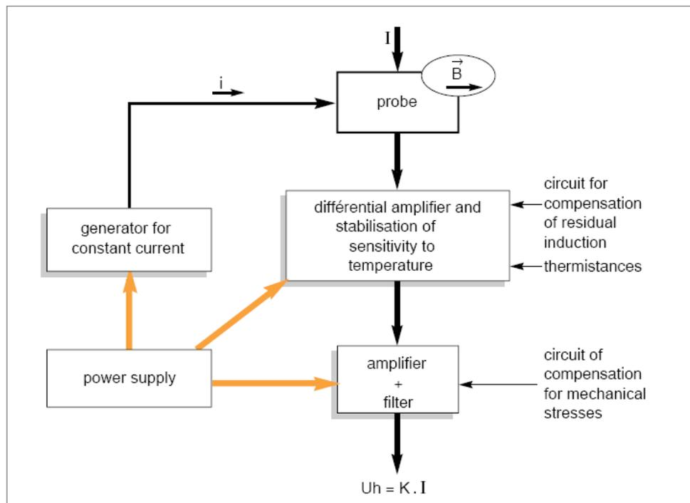
Figure 52 – Hall Effect Sensor (Courtesy of Schneider Electric – From II)
