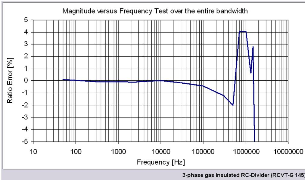
**Figure 39 – Measurements done on an RC voltage divider with a voltage level of 145 kV with a cable length of 150 m (courtesy of Trench Switzerland AG)**
