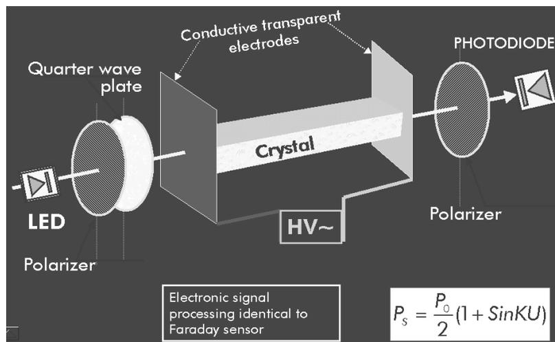
**Figure 29 – Basic design for a Pockels sensor (courtesy of Alstom Grid)**
