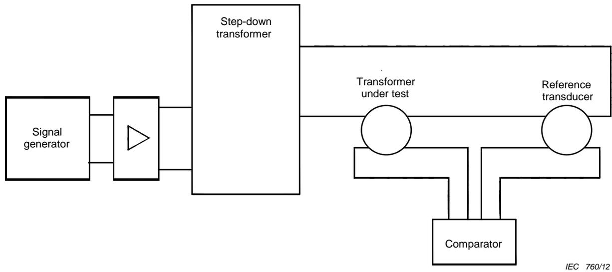
Figure 56 – Test circuit for CT frequency response test
