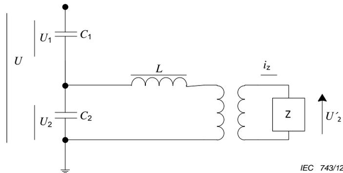
**Figure 20 – CVT: Equivalent circuit at power frequency**
