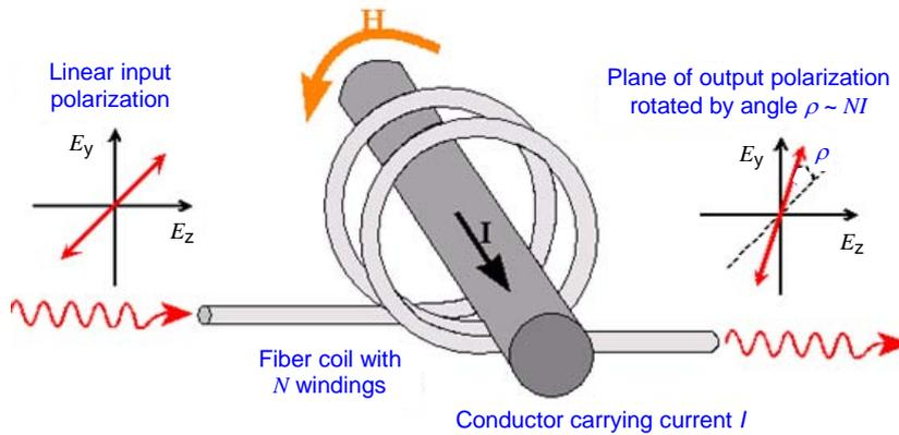
Figure 40 – Principle of optical CT measurement (from v))
