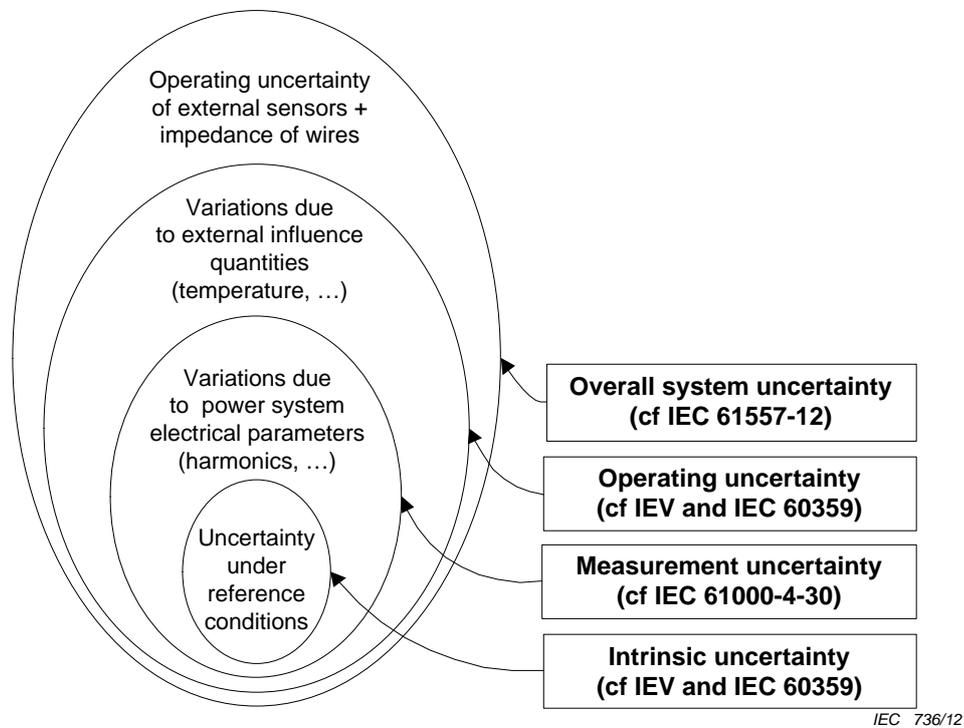
**Figure 2 – Contribution of instrument transformers in overall measurement uncertainty (from i), modified)**
