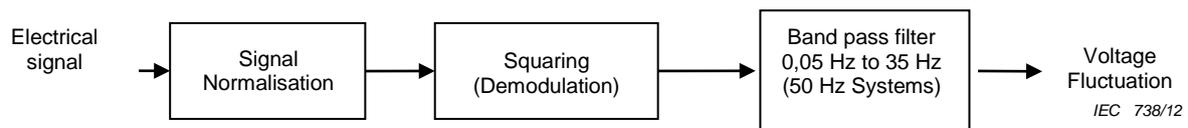
**Figure 4 – Demodulation within the IEC flickermeter**
