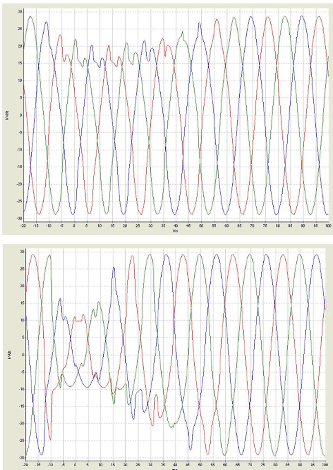
**Figure A.1 – Examples of “fake dips”, transients recorded at the secondary winding of MV voltage transformers due to voltage transformers saturation (courtesy of Italian distribution network monitoring system- QuEEN)**
