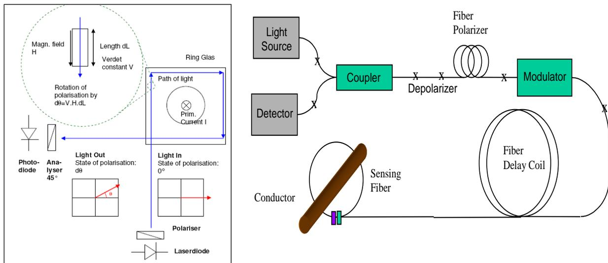
Figure 41 – Principle of optical CT measurement (Courtesy of Alstom Grid)
