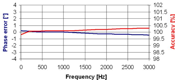
**Figure 38 – Frequency response of an RC voltage divider (courtesy of Trench Switzerland AG)**
