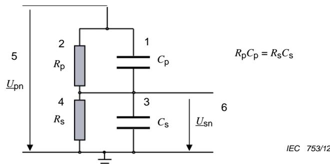
Figure 37 – Equivalent circuit of a balanced RC voltage divider (from x))
