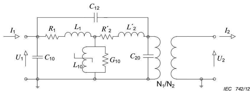
Figure 11 – Example of equivalent circuit for an inductive voltage/current transformer
