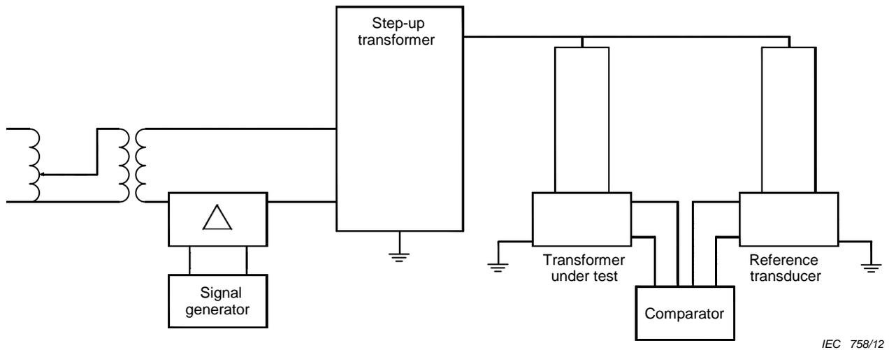
**Figure 54 – Test circuit for VT frequency response test**
