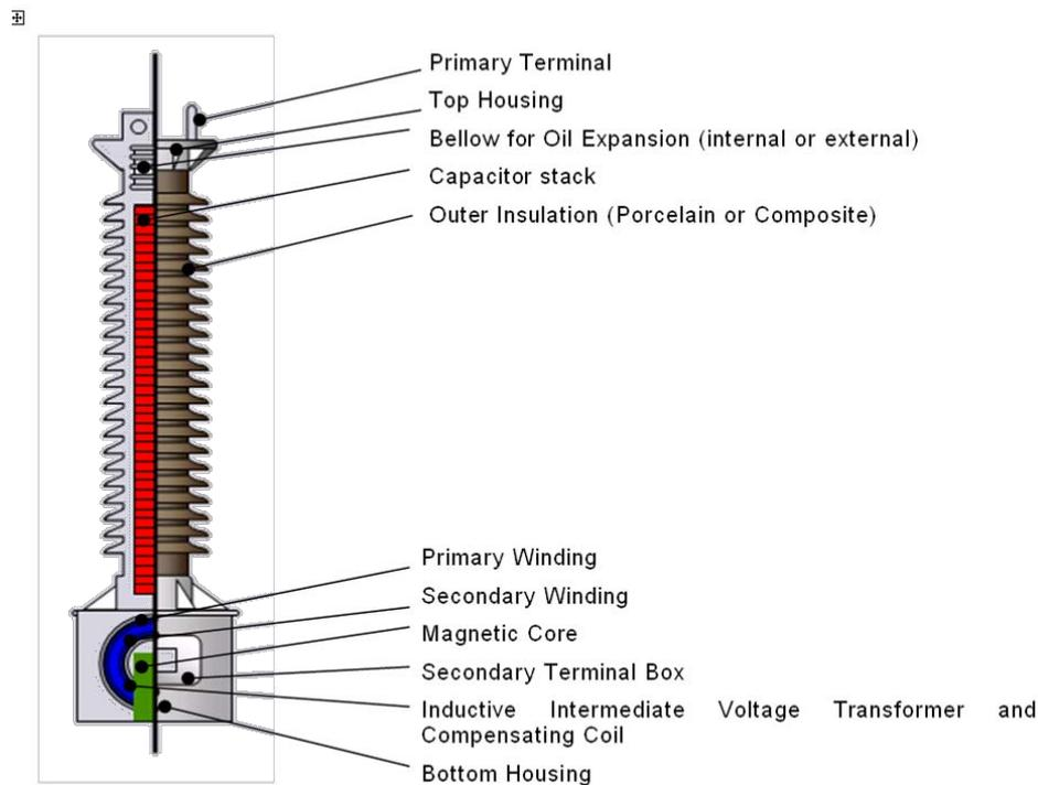
**Figure 19 – Cross-section view of a capacitive voltage transformer
