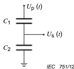
**Figure 35 – Electrical scheme of a capacitive voltage divider**
