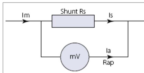
**Figure 46 – Electrical scheme of a shunt current measurement (Courtesy of Alstom Grid)**
