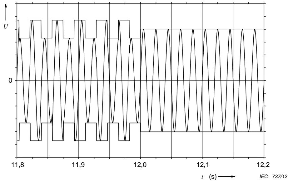
**Figure 3 – Example of voltage fluctuation causing flicker**
