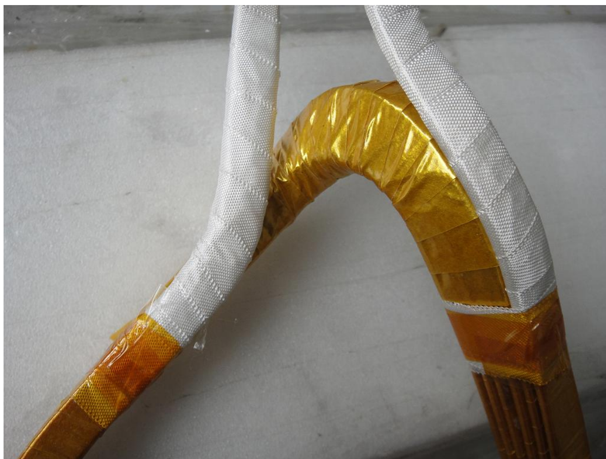
Figure B.6 – Close-up of formed coil's knuckle insulation
