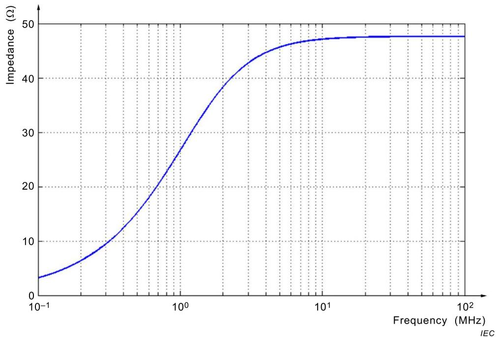
**Figure A.4 – Characteristics of the HV AN impedance**
