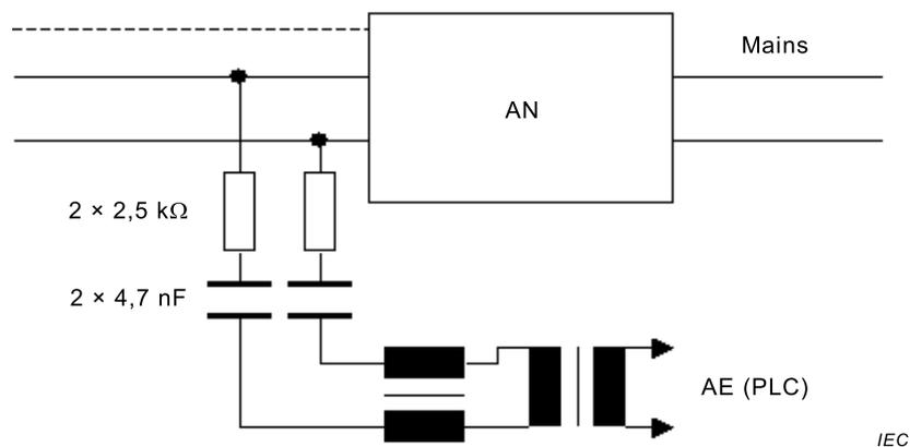
The value of the resistors depends on the allowed attenuation and the design impedance of the PLC modem (here: 40 dB attenuation, 100  $\Omega$  PLC design impedance).
