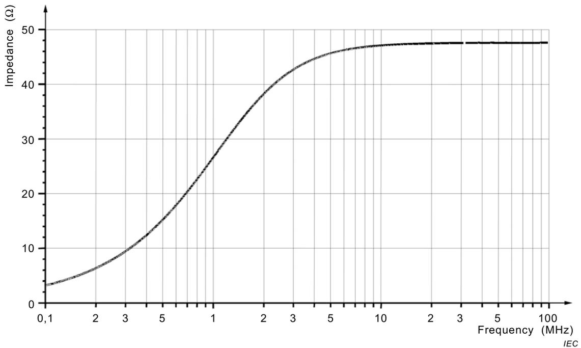
**Figure A.2 – Characteristics of the AN impedance**
