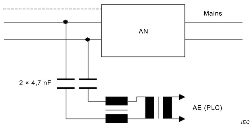
**Figure A.9 – Example of a circuit for immunity tests of PLC on AC or DC powerlines**
