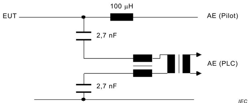
**Figure A.11 – Example of a circuit for immunity tests of PLC on control pilot line**
