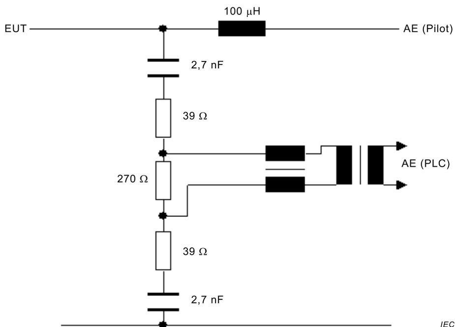
The values of the three resistors depend on the design impedance of the PLC modem connected on AE side. The values given in the schematic are valid for a design impedance of 100 Ω.
