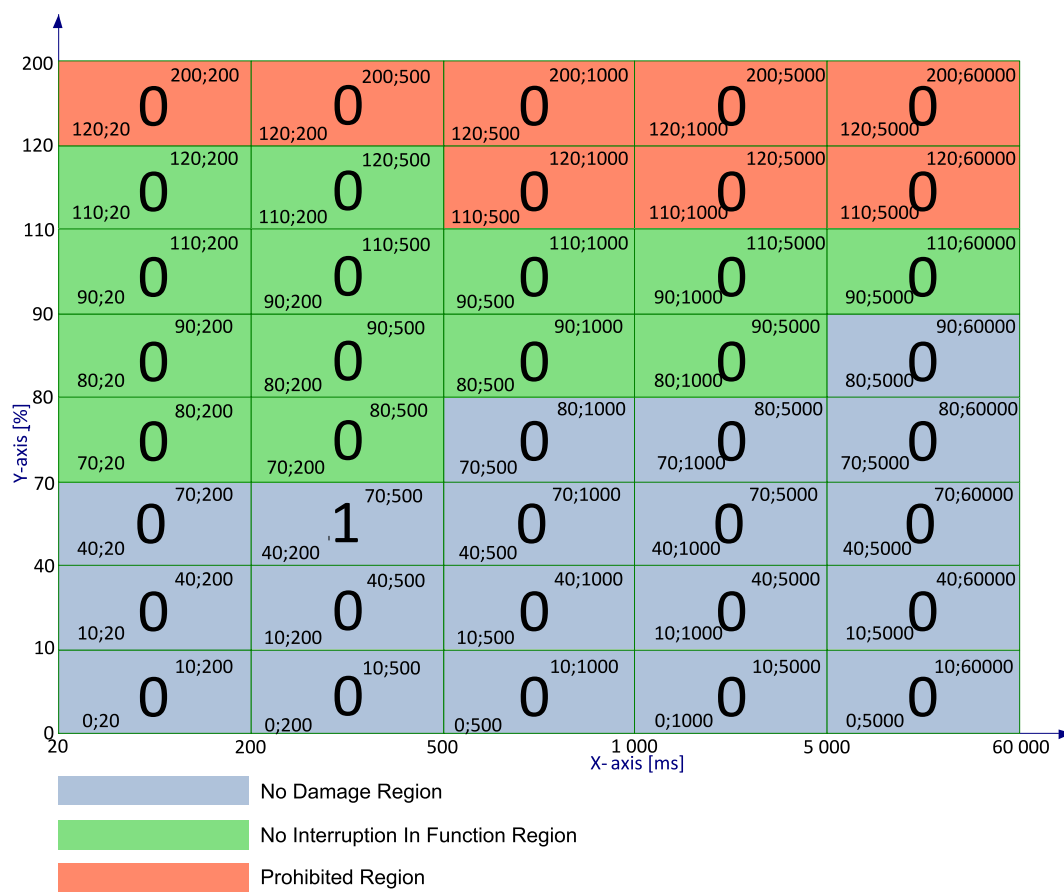
Figure 24 – Modelling of magnitude-duration table for voltage events with histogram HST
