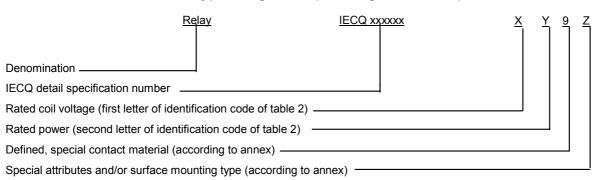
The coding of the monostable or bistable relay type shall be combined with the rated power of the coil, if applicable. The reference to the number and types of contacts shall be given on the front page of the specification.
