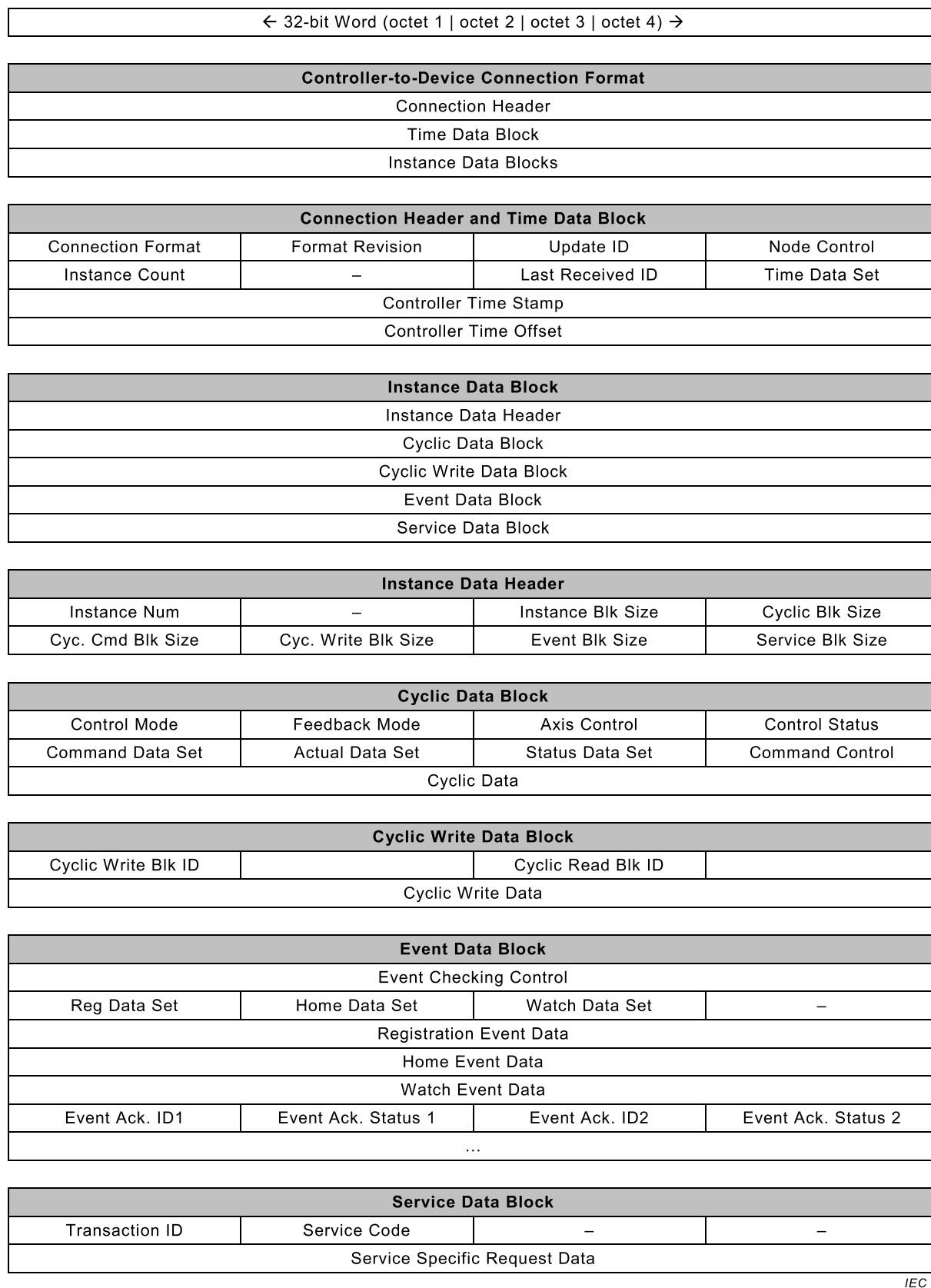
Figure 7 – Controller-to-Device I/O Connection Format (variable size)
