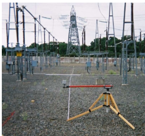
Figure 2 – Insulating tripod and offset rod for an electric field probe (photograph RTE)
