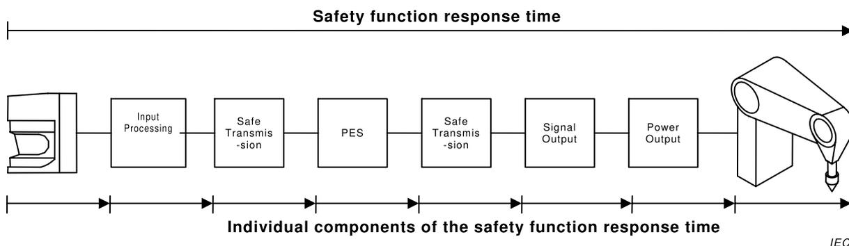
**Figure 6 – Example of safety function response time components**
