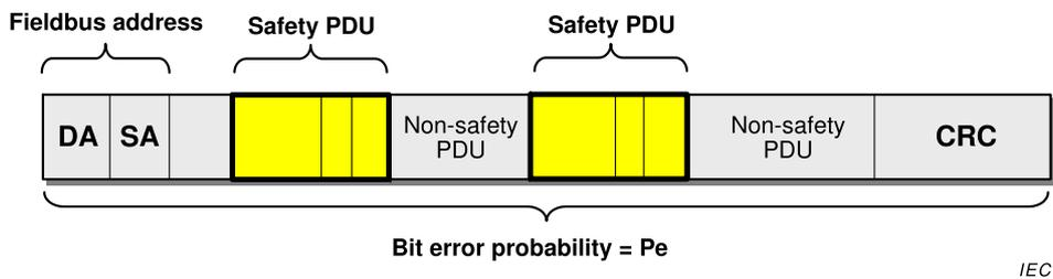
Figure E.1 – Example safety PDUs embedded in a fieldbus message
