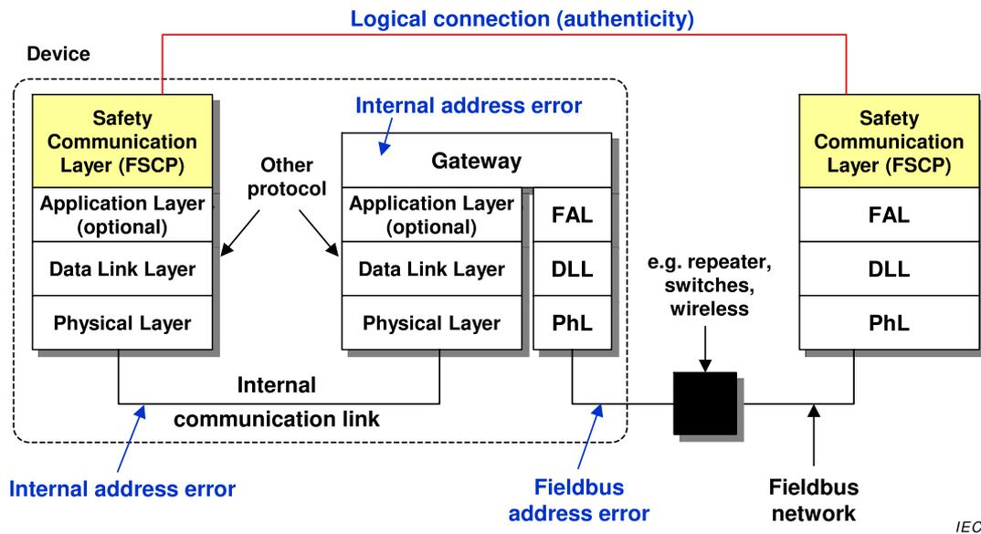
Figure F.3 – Fieldbus and internal address errors
