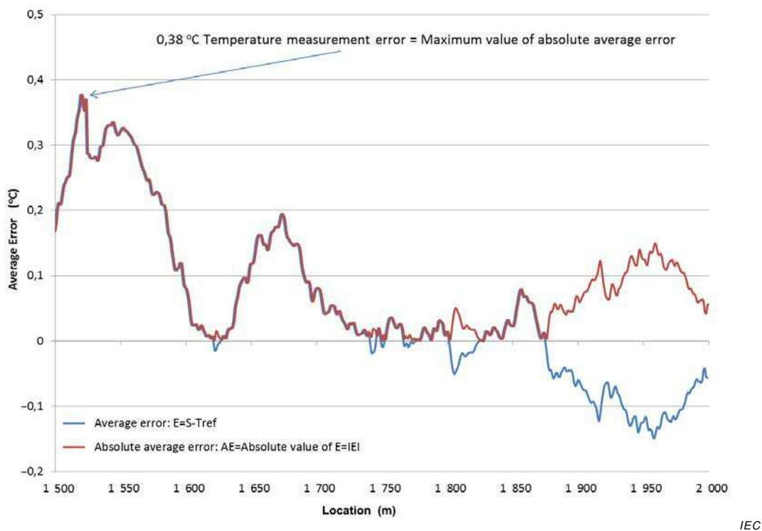
Figure 6 – Temperature measurement error calculation: steps 4 through 5
