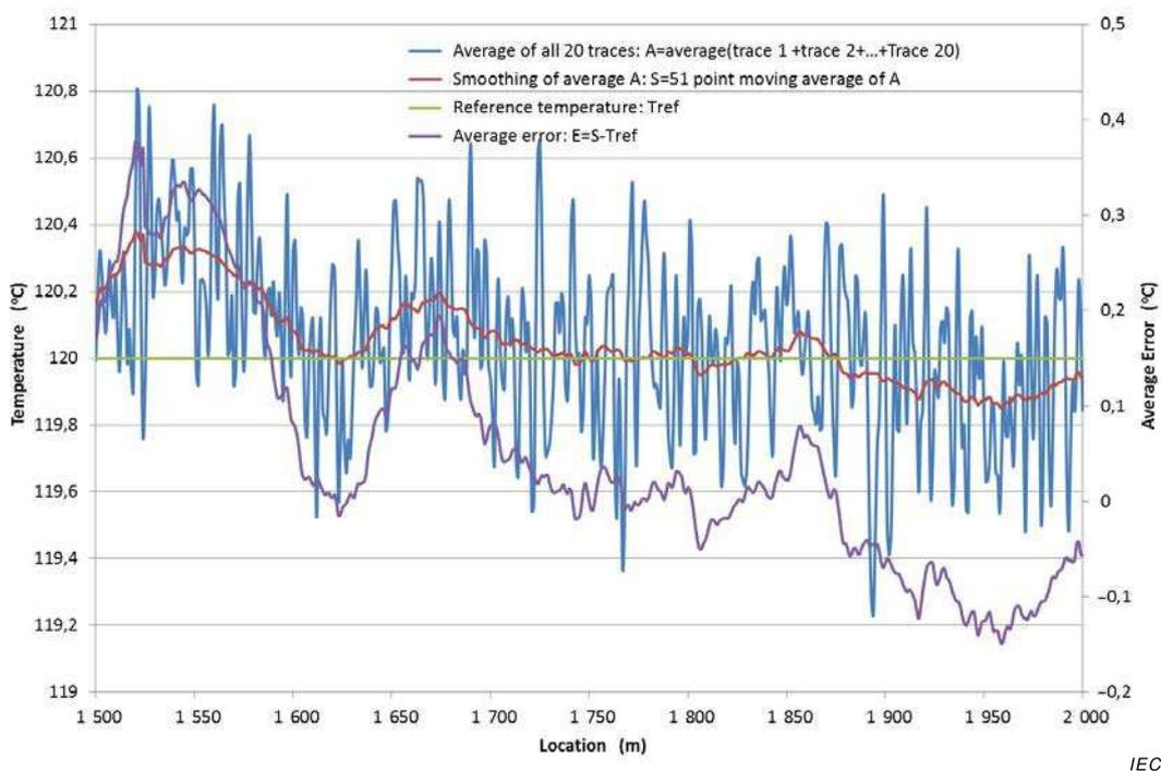
Figure 5 – Temperature measurement error calculation: steps 2 through 3
