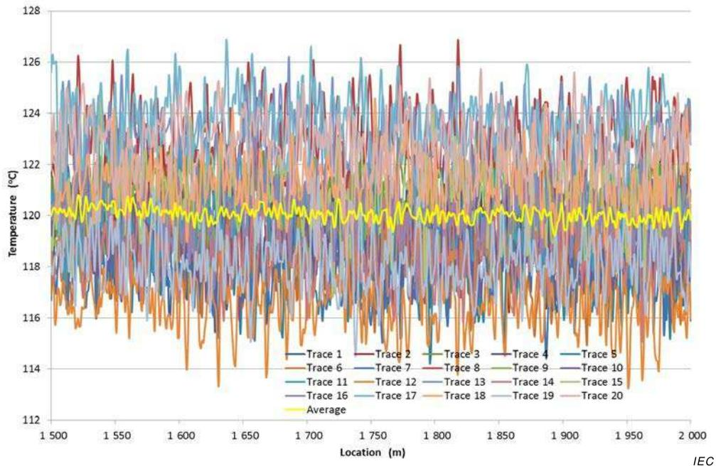
**Figure 4 – Temperature measurement error calculation: step 1**
