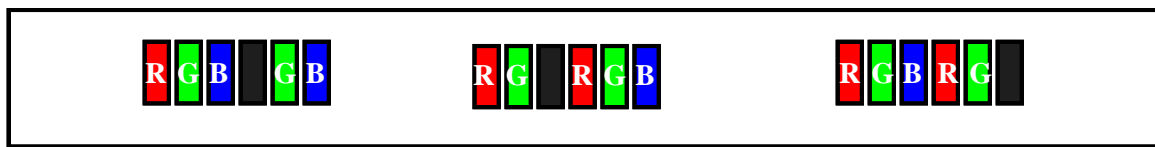
Figure 3 a) – One dark subpixel defect
