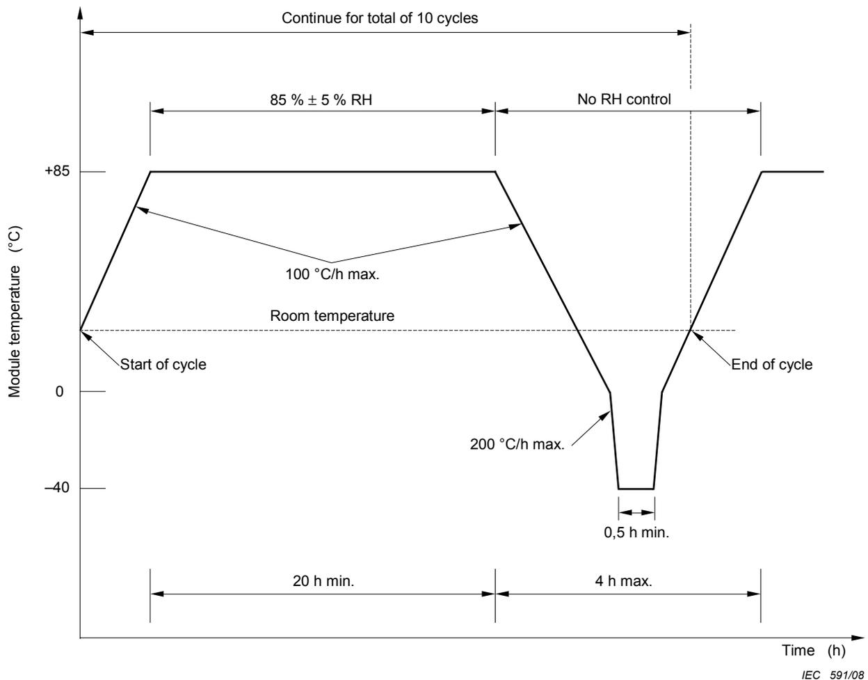
Figure 5 – Humidity-freeze cycle
